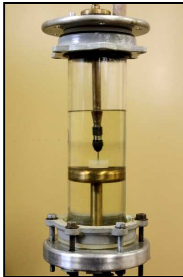
Figure S4. Insulation-oil-filled test cell loaded with a sample. Unwanted surface discharge can be avoided, which insures that all detected discharges are created internally in the sample.
