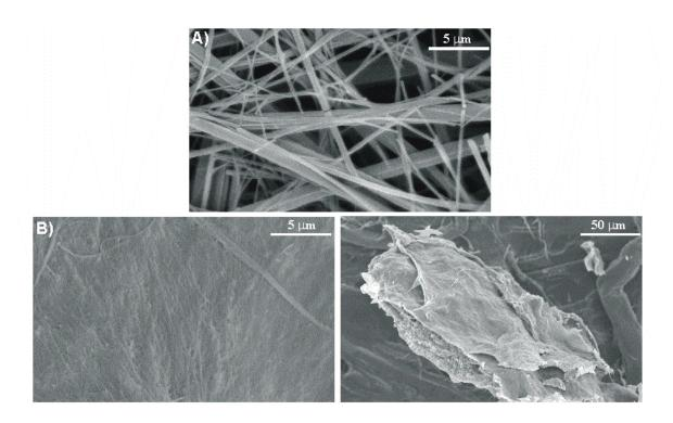
**Figure B**. SEM images at different magnifications of A) DF-OMe after heating at 403 K, B) DF DKP - (DF-OMe after heating at 463 K).
