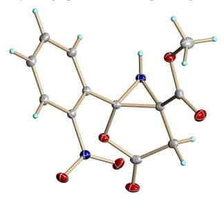
A clear colourless prism-like specimen of  $C_{12}H_{10}N_2O_6$ , approximate dimensions 0.10 mm × 0.28 mm × 0.50 mm, was used for the X-ray crystallographic analysis. The X-ray intensity data were measured on a Bruker Smart Apex2, CCD system equipped with a graphite monochromator and a MoK $\alpha$  fine focus sealed tube ( $\lambda = 0.71073$  Å). Data collection temperature was 150 K.
