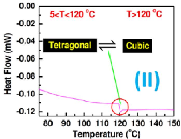
*Fig. I: Differential scanning calorimetric (DSC) scan of  $\text{BaTiO}_3$  nanoparticles showing distinct tetragonal to cubic phase transition at  $\sim 120^\circ\text{C}$*
