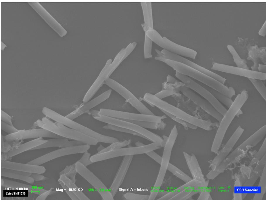
**Figure S9.** Electrodeposited polypyrrole micro-rods
