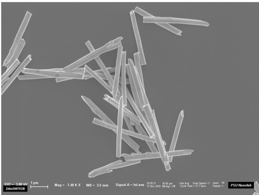
**Figure S7.** Electrodeposited Au micro-rods
