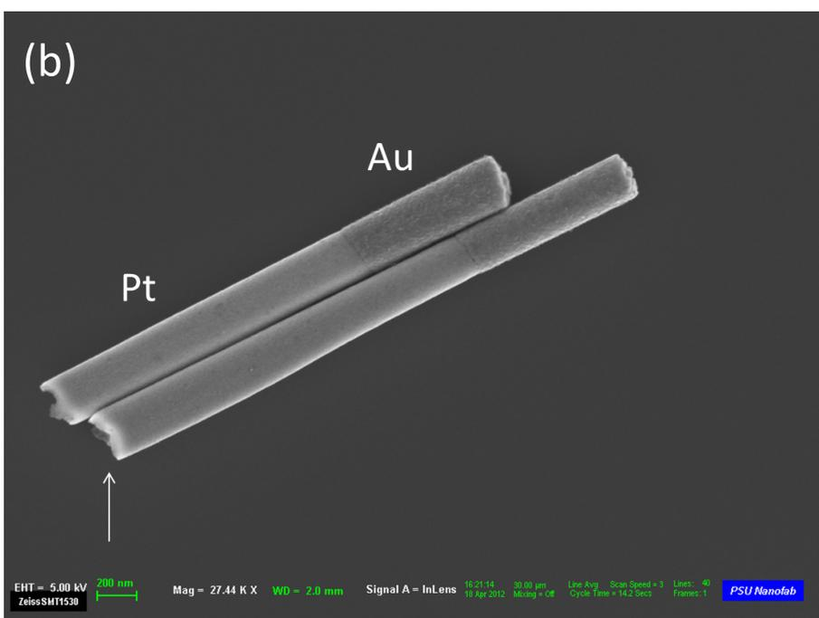
**Figure S4.** Electrodeposited AuPt (a) and PtAu (b) micro-rods. The arrow in (b) indicates the concave feature at the Pt end.
