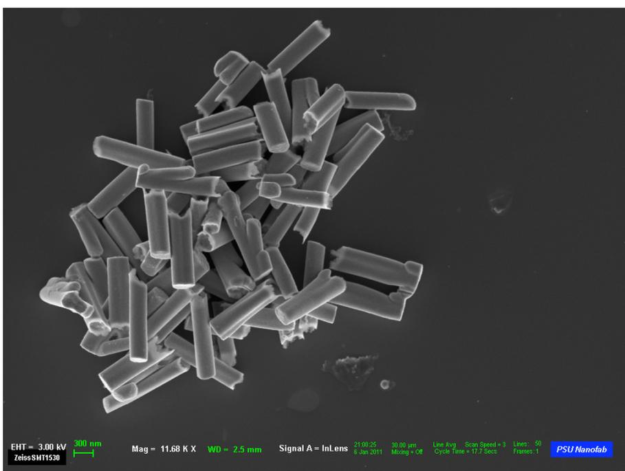
**Figure S6.** Electrodeposited Ru micro-rods
