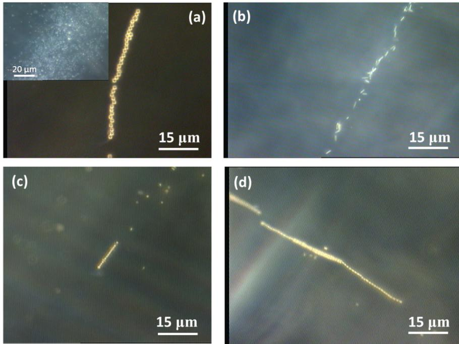
**Figure S11** Chains formed by different samples in an acoustic field. (a) 2  $\mu\text{m}$  polystyrene microparticles (inset: 470 nm polystyrene particles); (b) polypyrrole micro-rods; (c) gold microspheres; (d) gold micro-rods
