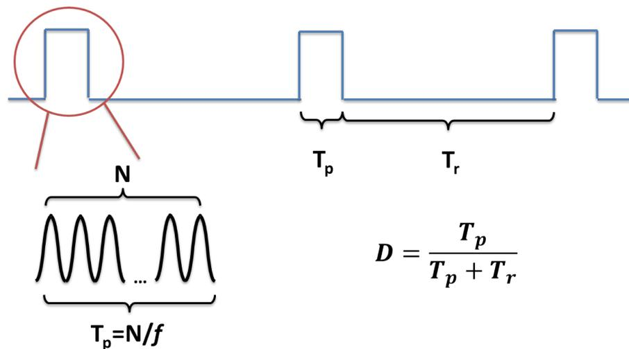
**Figure S12.** An illustration of the parameters used in the pulsed-mode experiments.
