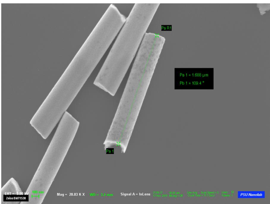
**Figure S8.** Electrodeposited Pt micro-rods
