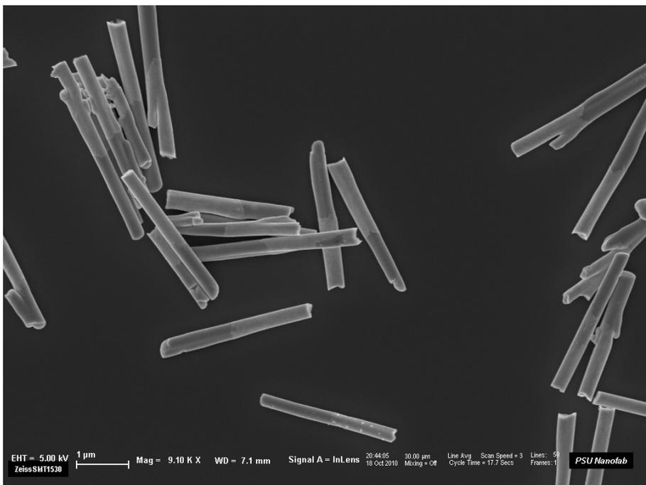
**Figure S5.** Electrodeposited AuRu micro-rods
