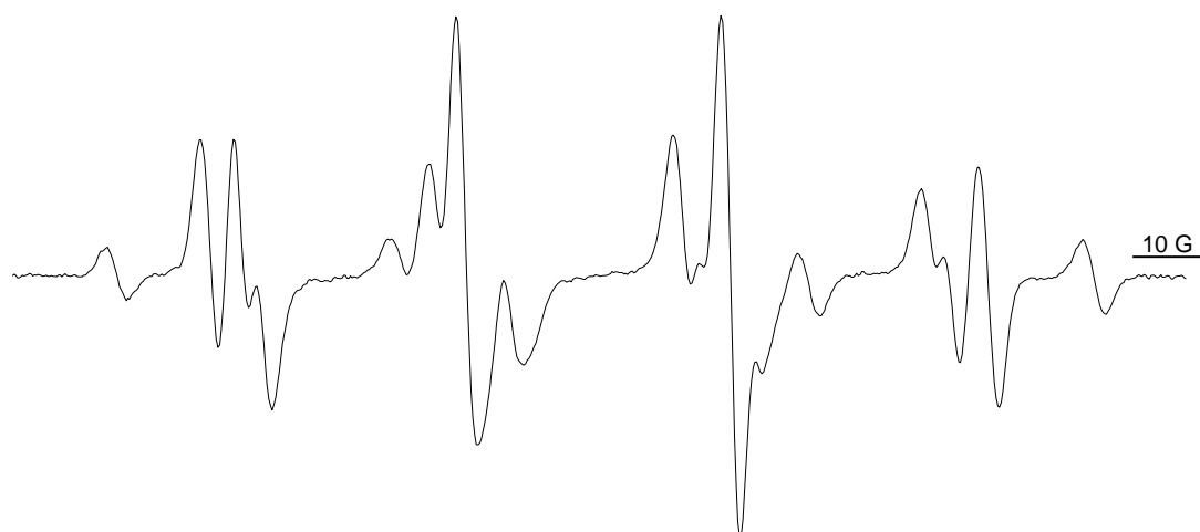
Figure S7. EPR spectrum of procarbazine-derived radicals at zero time catalyzed by 2 \mu M HRP.
