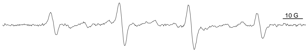
Figure S8. EPR spectrum of phenylhydrazine-derived radicals at zero time catalyzed by 0.5 \mu\text{M} HRP
