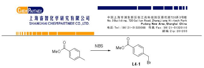
A mixture of methyl 4-methylbenzoate (50.0 g, 0.333 mol), NBS (53.4 g, 0.300 mol) and AIBN (5 g) in  $CCl_4$  (1000 mL) was refluxed for 7h. Then the mixture was filtered and concentrated to afford L4-1 (76.5 g) as light yellow oil in 100 % yield. The crude product was used in the next step without further purification.
