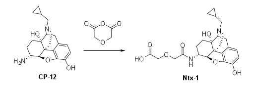
To a solution of **CP-12** (60 mg, 0.175 mmol) in THF (10 mL) was added diglycolic anhydride (28 mg, 0.245 mmol) one portion under ice-salt bath. The reaction was stirred overnight at r.t. and then concentrated to give **Ntx-1** (82 mg) as gray solid in quantitative yield. The crude product was used in the next step without further purification.
