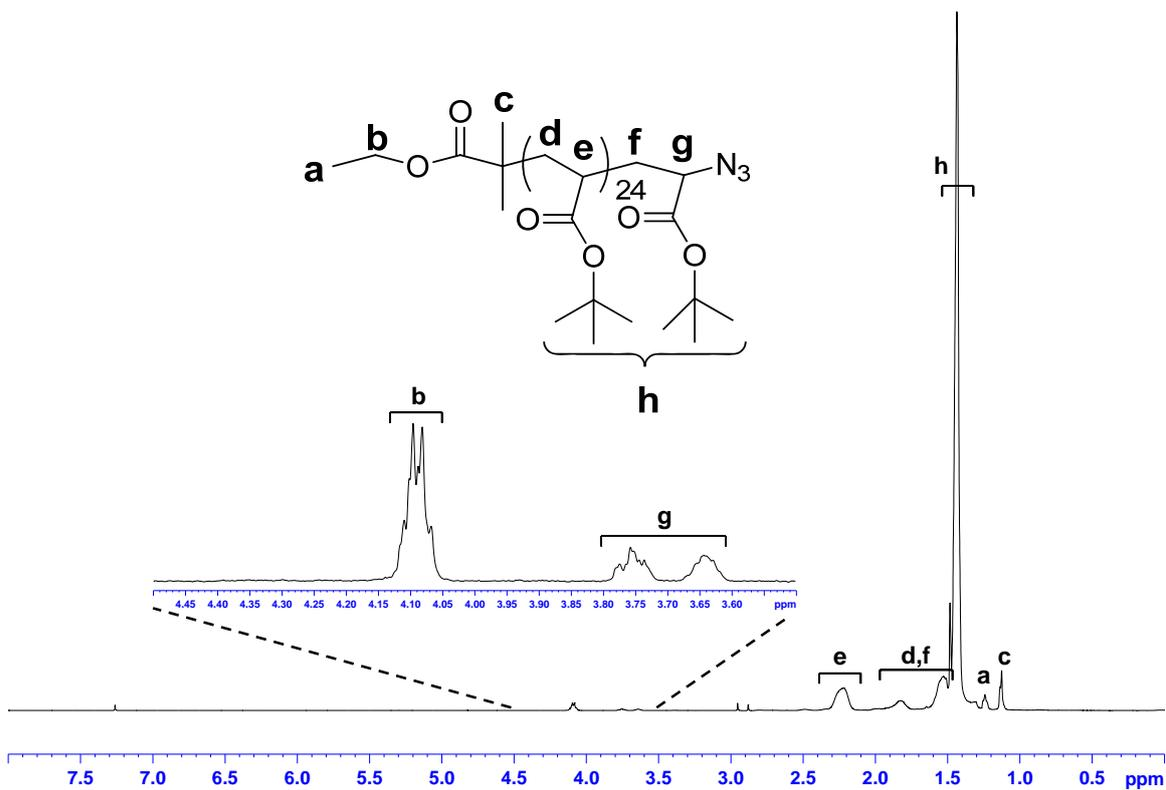
Figure S18: <sup>1</sup>H 1D DOSY NMR analysis of P<sup>t</sup>BA<sub>25</sub>-N<sub>3</sub> (7).
