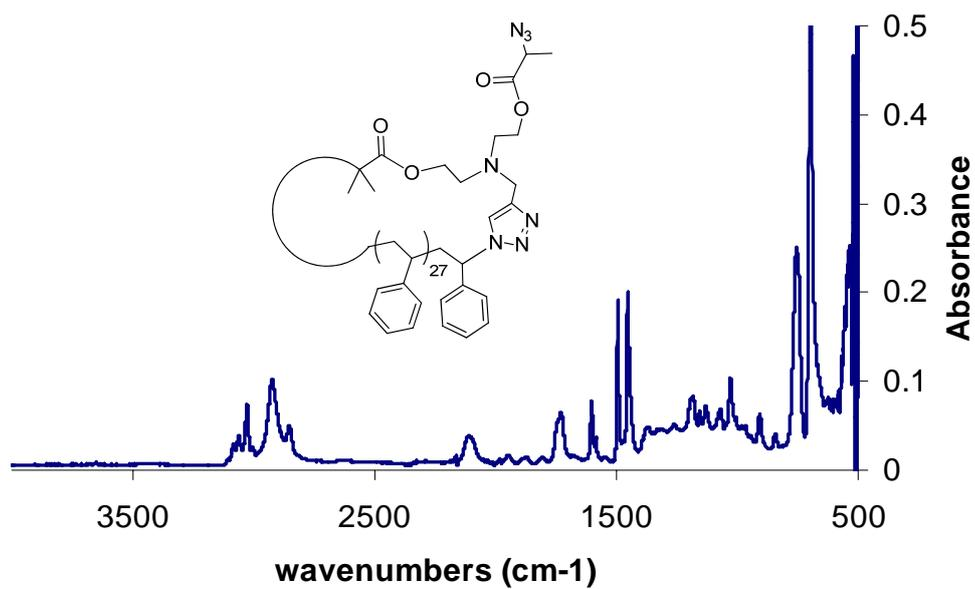
Figure S14: ATR-FTIR spectra of c-PSTY<sub>28</sub>-N<sub>3</sub> (5)
