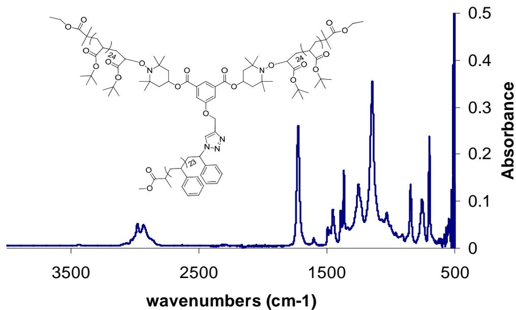
Figure S31: ATR-FTIR spectra of P(STY<sub>24</sub>-b-(<sup>t</sup>BA<sub>25</sub>)<sub>2</sub>) 12
