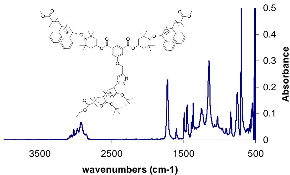
Figure S27: ATR-FTIR spectra of P(<sup>1</sup>BA<sub>25</sub>-b-(STY<sub>24</sub>)<sub>2</sub>) **10**
