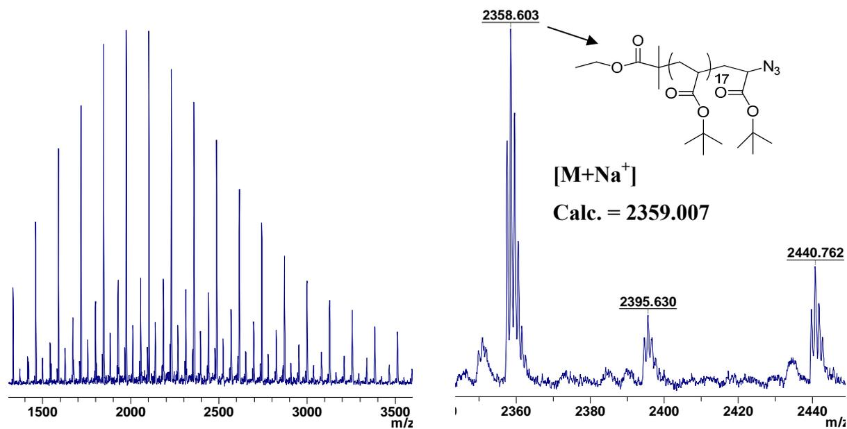
**Figure S20:** MALDI-ToF mass spectrum of P<sup>t</sup>BA<sub>25</sub>-N<sub>3</sub> (7) with Na salt as cationization agent from a DCTB matrix in reflectron mode: (left) full molecular weight distribution, (right) isotopic resolution of peaks.
