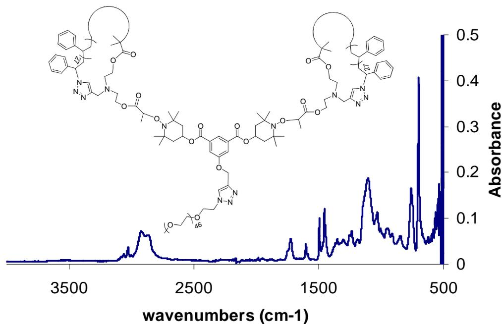
Figure S37: ATR-FTIR spectra of P(EG<sub>47</sub>-b-(cSTY<sub>28</sub>)<sub>2</sub>) 15
