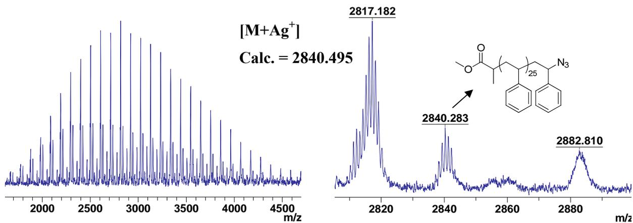
**Figure S6:** MALDI-ToF mass spectrum of PSTY<sub>24</sub>-N<sub>3</sub> (**3**) with Ag salt as cationization agent from a DCTB matrix in reflectron mode: (left) full molecular weight distribution, (right) isotopic resolution of peaks.
