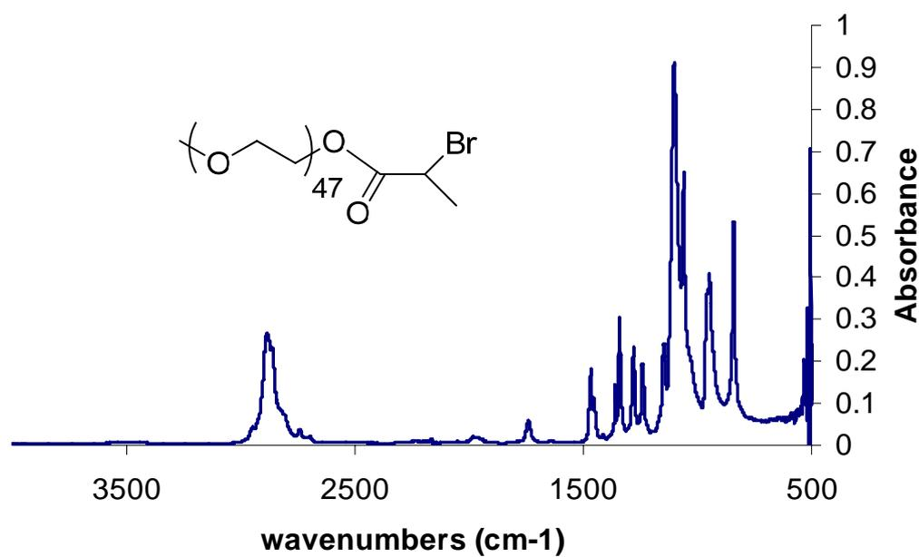
Figure S22: ATR-FTIR spectra of PEG<sub>47</sub>-Br (8).
