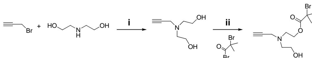
**Scheme S1:** Synthesis of alkyne(hydroxyl) ATRP initiator. (i)  $K_2CO_3$ , acetone, reflux for 24 h; (ii) TEA, THF at 0 °C.
