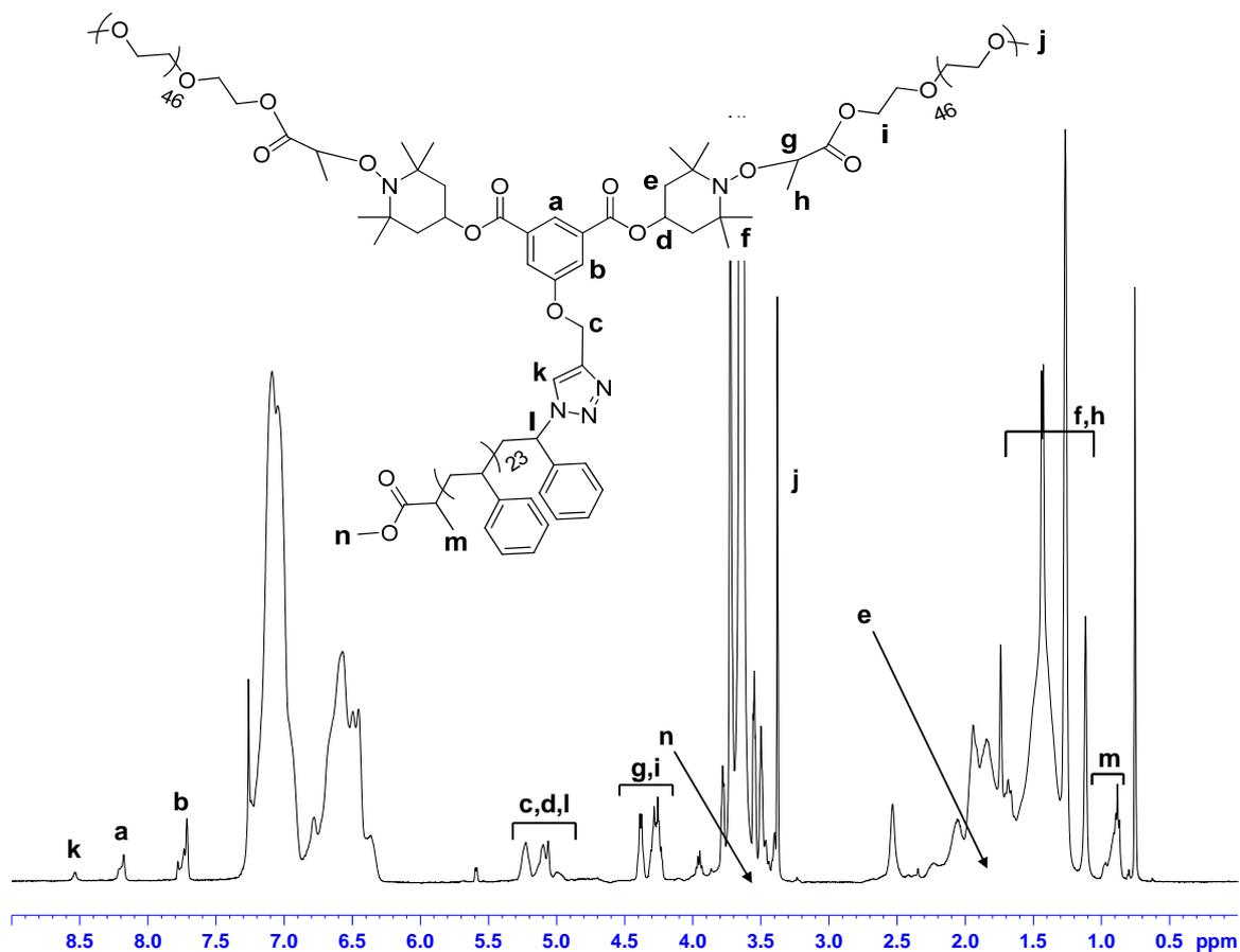
Figure S32: <sup>1</sup>H 1D DOSY NMR analysis of P(STY<sub>24</sub>-b-(EG<sub>47</sub>)<sub>2</sub>) 13
