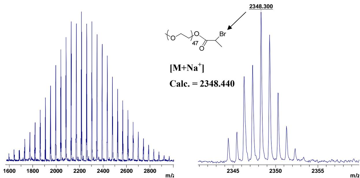
**Figure S23:** MALDI-ToF mass spectrum of PEG<sub>47</sub>-Br (**8**) with Na salt as cationization agent from a 2-(4'-Hydroxybenzeneazo)benzoic acid (HABA) matrix in reflectron mode: (left) full molecular weight distribution, (right) isotopic resolution of peaks.
