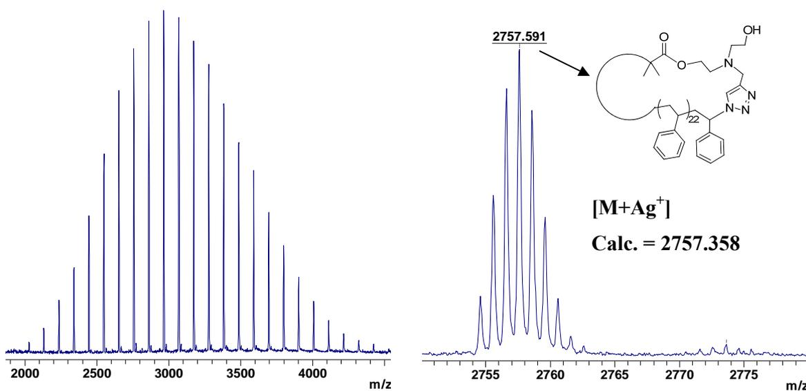
**Figure S10:** MALDI-ToF mass spectrum of c-PSTY<sub>28</sub>-OH with Ag salt as cationization agent from a DCTB matrix in reflectron mode: (left) full molecular weight distribution, (right) isotopic resolution of peaks.
