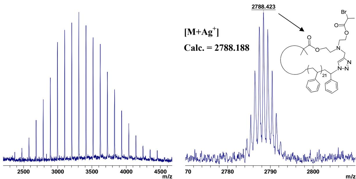
Figure S12: MALDI-ToF mass spectrum of c-PSTY<sub>28</sub>-Br with Ag salt as cationization agent from a DCTB matrix in reflectron mode: (left) full molecular weight distribution, (right) isotopic resolution of peaks.
