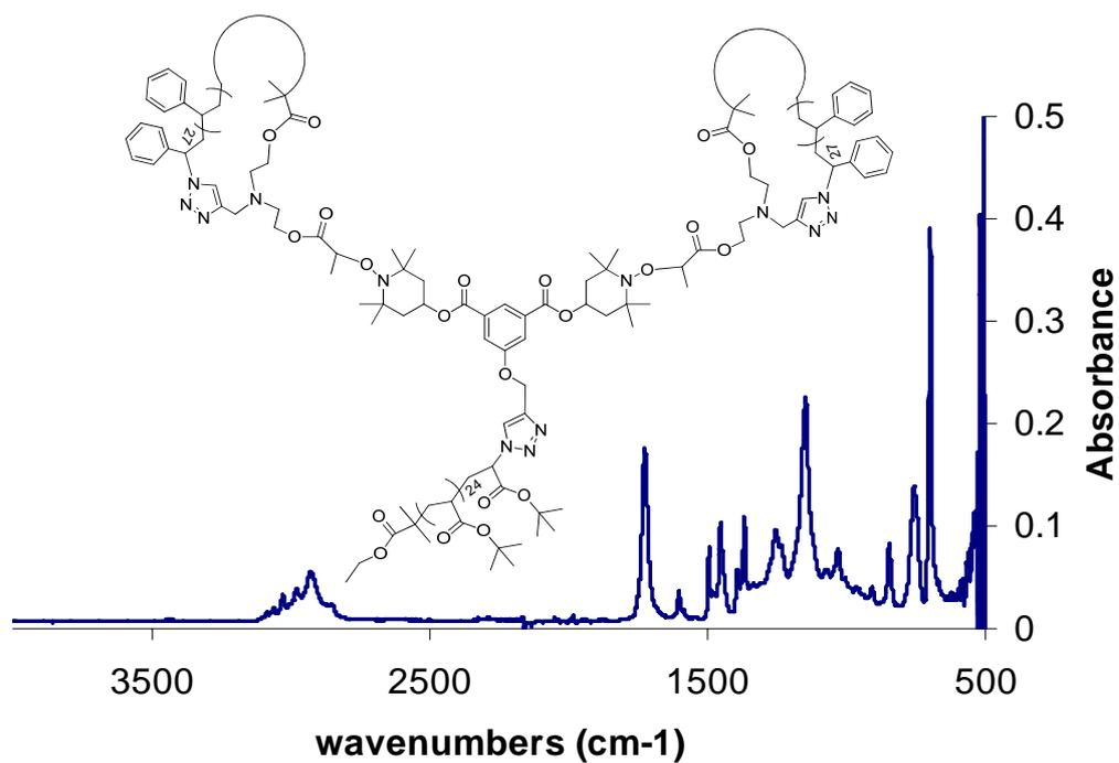
Figure S35: ATR-FTIR spectra of P(<sup>t</sup>BA<sub>25</sub>-b-(cSTY<sub>28</sub>)<sub>2</sub>) 14
