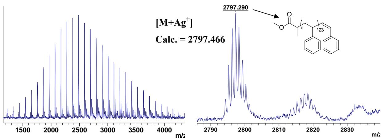
**Figure S3:** MALDI-ToF mass spectrum of PSTY<sub>24</sub>-Br (2) with Ag salt as cationization agent from a DCTB matrix in reflectron mode: (left) full molecular weight distribution, (right) isotopic resolution of peaks.
