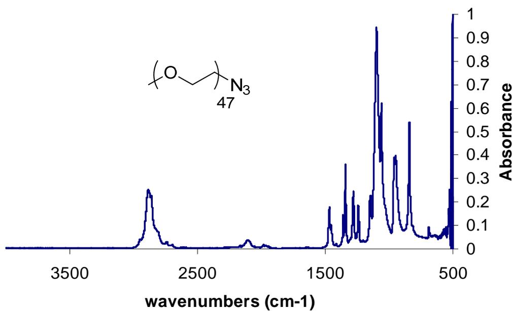
Figure S25: ATR-FTIR spectra of PEG<sub>47</sub>-N<sub>3</sub> (9)
