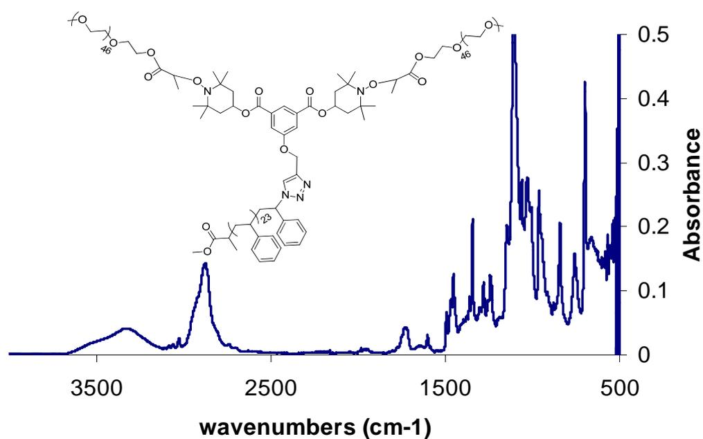
Figure S33: ATR-FTIR spectra of P(STY<sub>24</sub>-b-(EG<sub>47</sub>)<sub>2</sub>) 13
