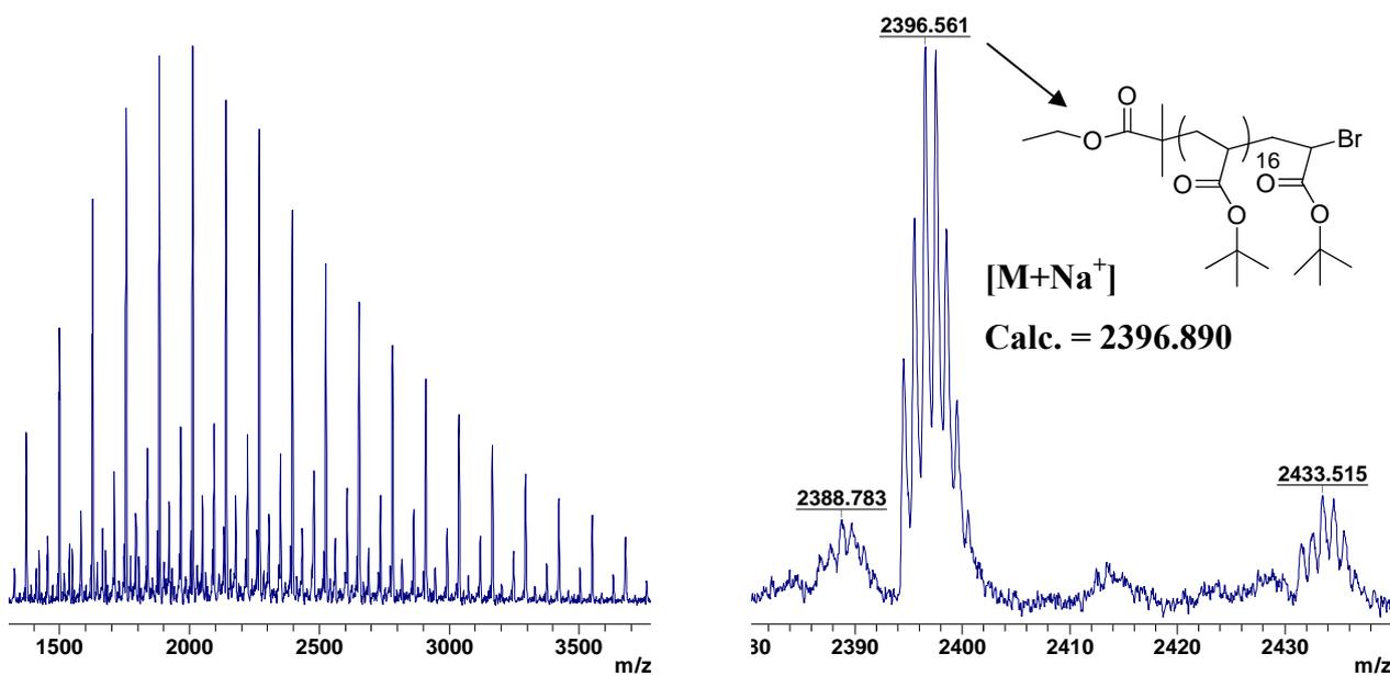
**Figure S17:** MALDI-ToF mass spectrum of P<sup>t</sup>BA<sub>25</sub>-Br **6** with Na salt as cationization agent from a DCTB matrix in reflectron mode: (left) full molecular weight distribution, (right) isotopic resolution of peaks.
