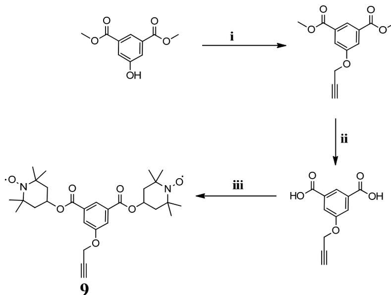
(i)  $K_2CO_3$ , propargyl bromide, 18-c-6, acetone, reflux 24 h; (ii) 2M NaOH, MeOH/acetone (60:40 v/v), RT, 24 h; (iii) TEMPO- $\equiv$ , EDC.HCl, DMAP, DMF, 0 °C – RT, 48 h.
