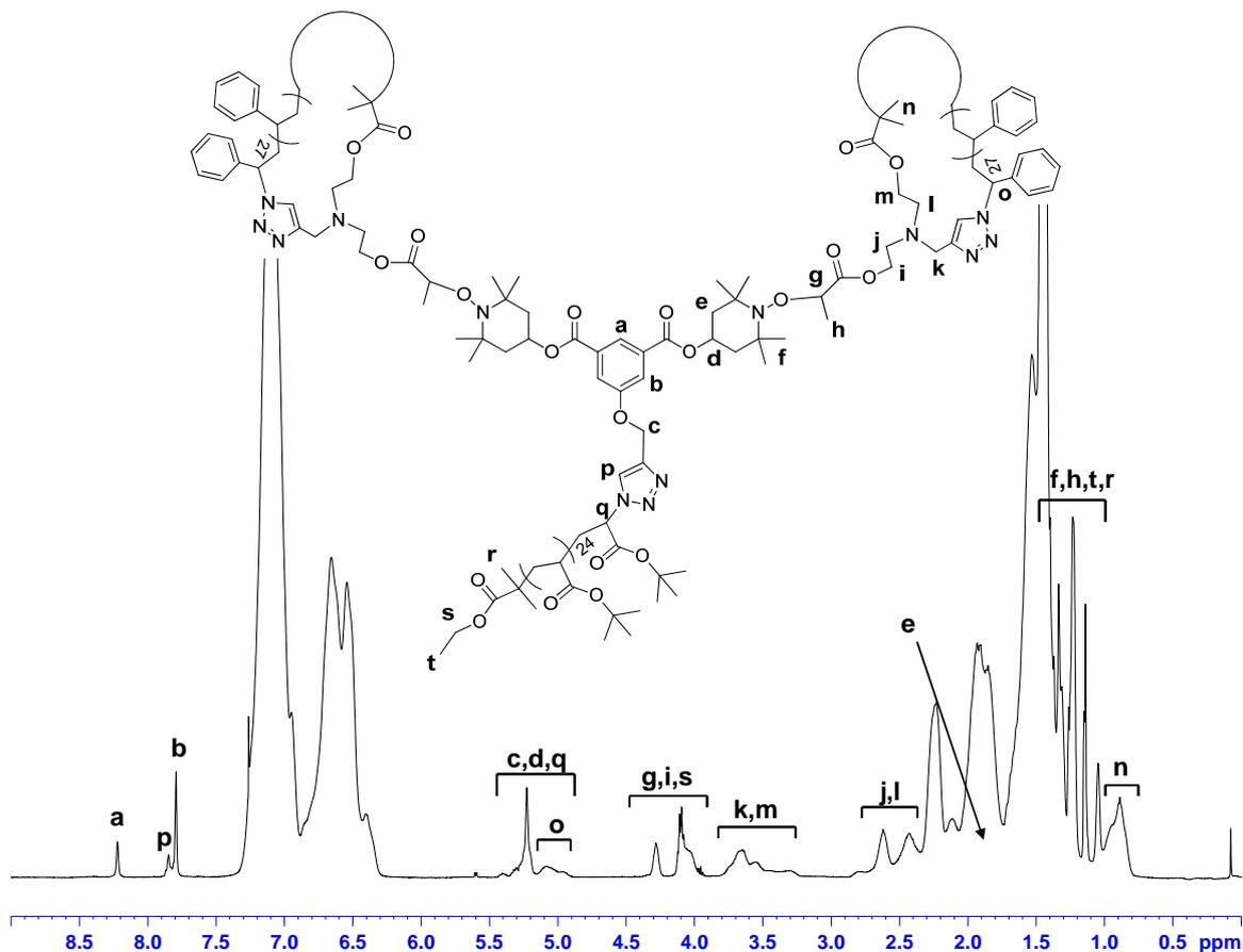
Figure S34: <sup>1</sup>H 1D DOSY NMR analysis of P(<sup>t</sup>BA<sub>25</sub>-b-(cSTY<sub>28</sub>)<sub>2</sub>) 14
