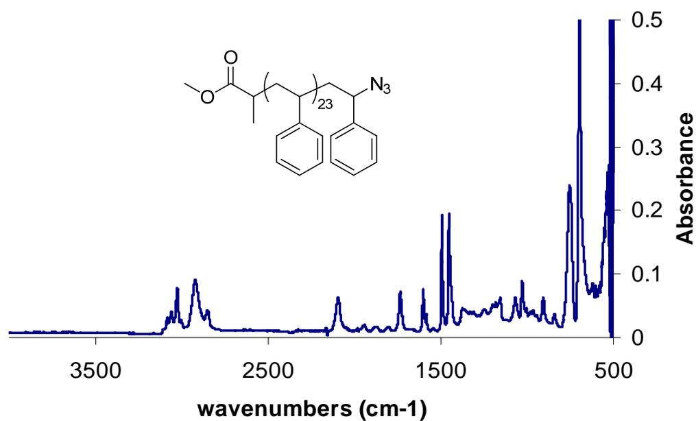
Figure S5: ATR-FTIR spectra of PSTY<sub>24</sub>-N<sub>3</sub> (3)
