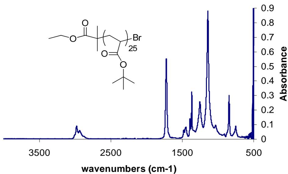
Figure S16: ATR-FTIR spectra of P<sup>t</sup>BA<sub>25</sub>-Br (6)
