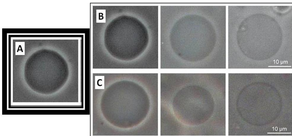
**Figure S1.** Representative transmission microscopy images of different DOPC giant unilamellar vesicles (GUVs) treated with a single nanopulse. The images were collected before (A) or a couple of minutes after the application of a 10 ns pulse of 3.2kV/mm (B) or of 5.8kV/mm (C). Note the fading contrast between the internal media (sucrose 240 mM) and external media (glucose 260 mM), indicative of an exchange of sugars across the lipid membranes and therefore an electroporation of the vesicles.
