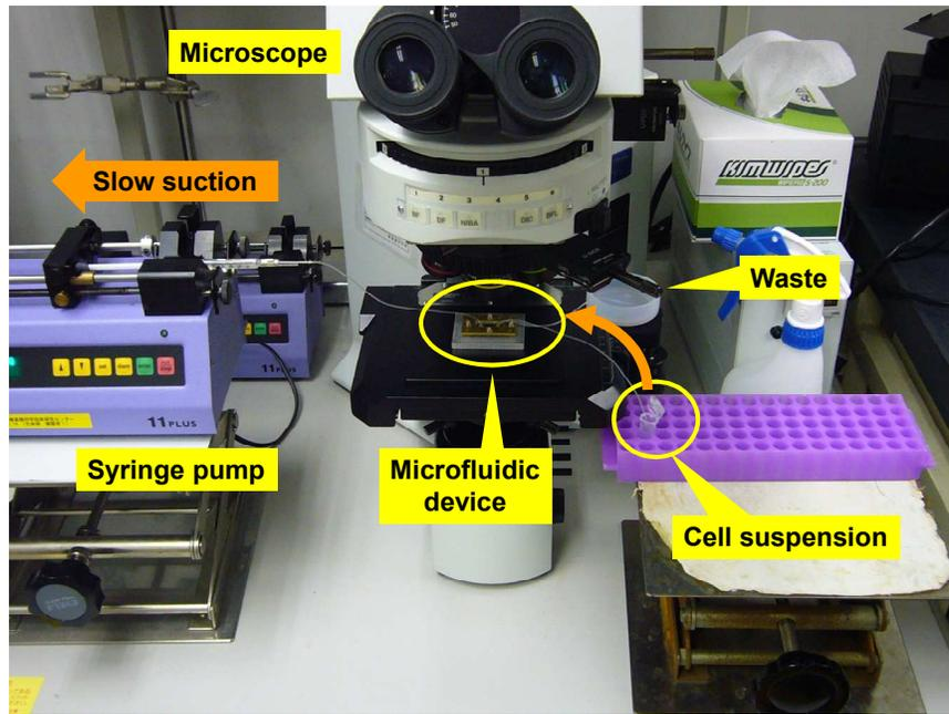
**Figure S3.** Whole system including microfluidic device, microscope, and syringe pump.
