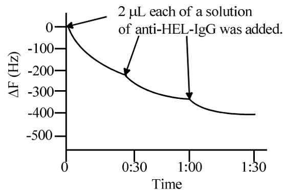
**Figure S2.** 27 MHz QCM results for the interaction between anti-HEL-IgG and HEL. Time course for frequency change of QCM. The association constant  $K_a$  was estimated to be  $1.35 \times 10^8$  [ $\text{M}^{-1}$ ] (dissociation constant  $K_d = 7.4$  nM) from these curves (Ref. 54 in the text).
