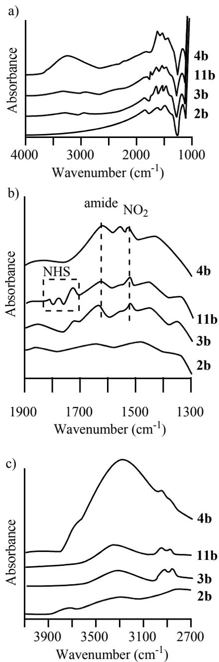
**Figure S1.** FTIR-ATR spectra of IgG-modified porous Si **4b** in the 4000 to 1000  $\text{cm}^{-1}$  (a), 1900 to 1300  $\text{cm}^{-1}$  (b) and 4000 to 2700  $\text{cm}^{-1}$  (c)
