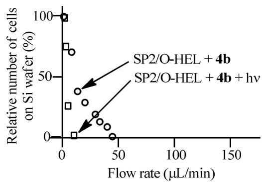
**Figure S6.** Relative numbers of cells observed on the porous Si wafer with increasing PBS buffer flow rate. Relative numbers of SP2/O-HEL on porous silicon wafer **4b** before or after photoirradiation are shown as open circles and open squares, respectively.
