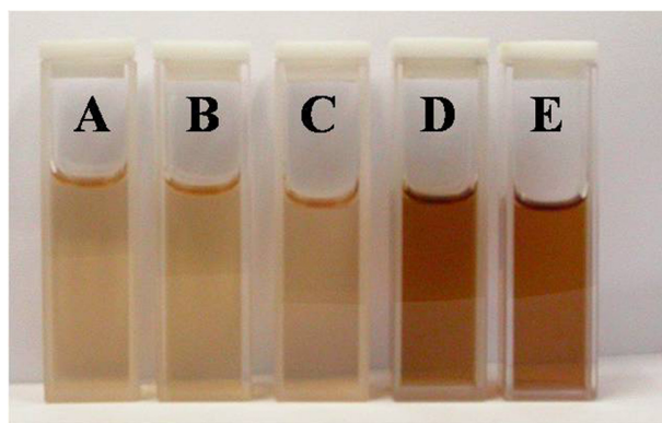
Figure S3. Bright-field photographs of PPPB solutions (0.2mg/mL) in DMF without and with addition of anions at the pyridinium/anion molar ratio of 1:1. (A: PPPB, B: PPPB+NaCl, C: PPPB+NaNO 3 , D: PPPB+CH 3 COONa, E: PPPB+HCOONa)
