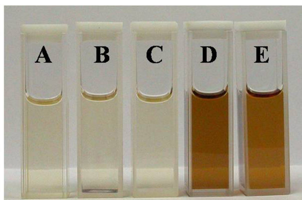
Figure S3. Bright-field photographs of PPPB solutions (0.2mg/mL) in DMF without and with addition of anions at the pyridinium/anion molar ratio of 1:1. (A: PPPB, B: PPPB+NaCl, C: PPPB+NaNO 3 , D: PPPB+CH 3 COONa, E: PPPB+HCOONa)
