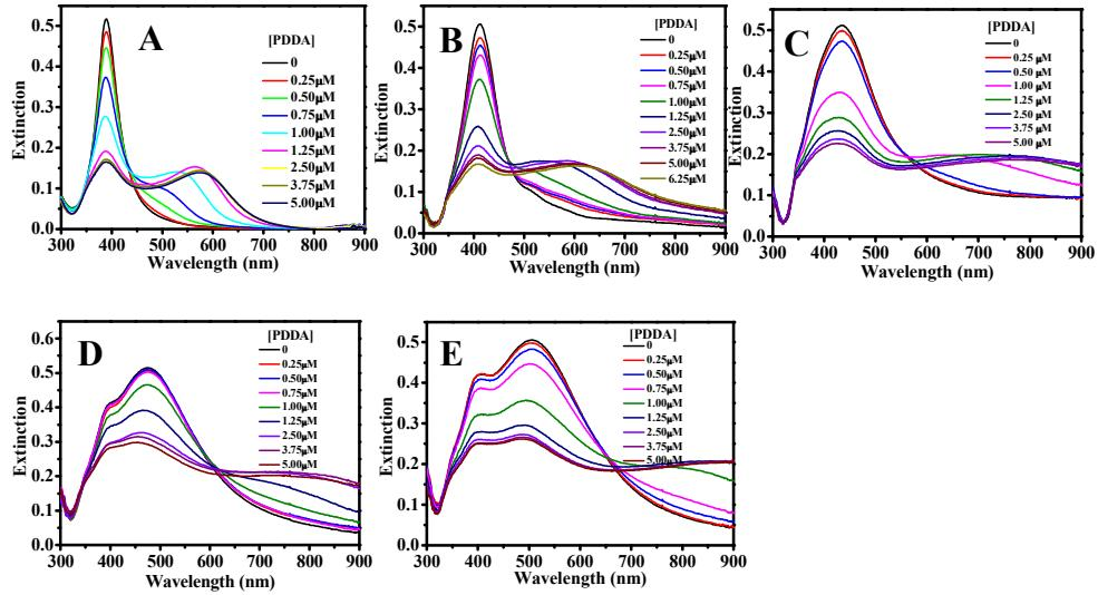
**Figure S2.** UV-Vis extinction spectra of (A) 15 nm, (B) 30 nm, (C) 50 nm, (D) 75 nm and (E) 100 nm Ag NSs in the presence of different amounts of PDDA.
