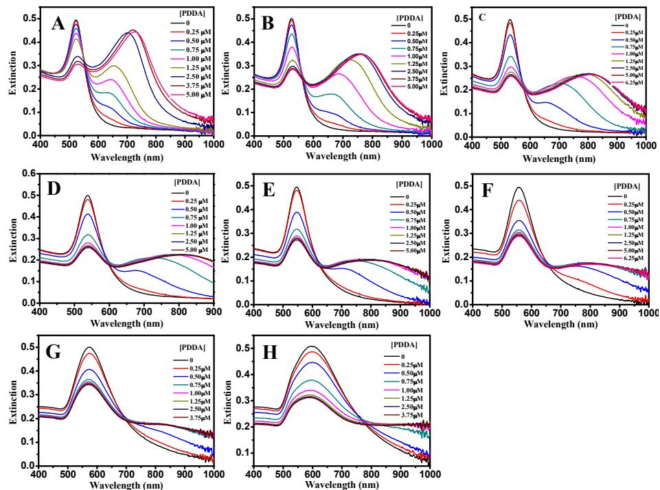
**Figure S1.** UV-Vis extinction spectra of (A) 20 nm, (B) 30 nm, (C) 40 nm, (D) 55 nm, (E) 80 nm, (F) 95 nm, (G) 110 nm and (H) 120 nm Au NSs in the presence of different amounts of PDDA.
