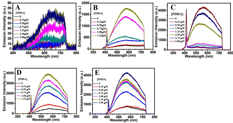
**Figure S4.** TPPL spectra of (a) 15 nm, (b) 30 nm, (c) 50 nm, (d) 75 nm and (e) 100 nm Ag NSs in presence of different amounts of PDDA.
