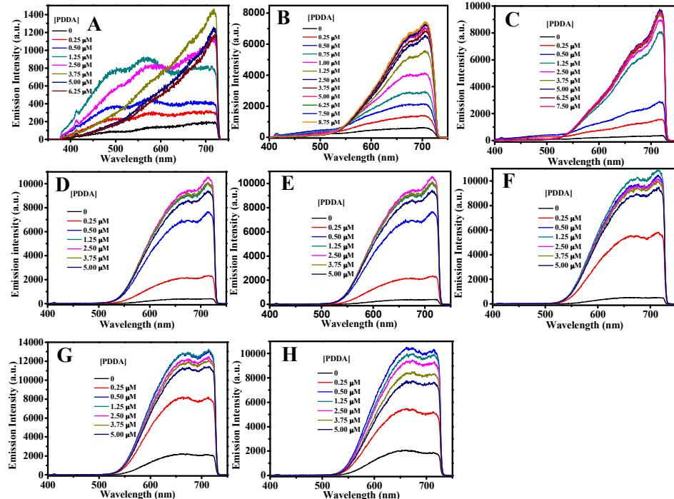
**Figure S3.** TPPL spectra of (a) 20 nm, (b) 30 nm, (c) 40 nm, (d) 55 nm, (e) 80 nm, (f) 95 nm, (g) 110 nm and (h) 120 nm Au NSs in the presence of different amounts of PDDA.
