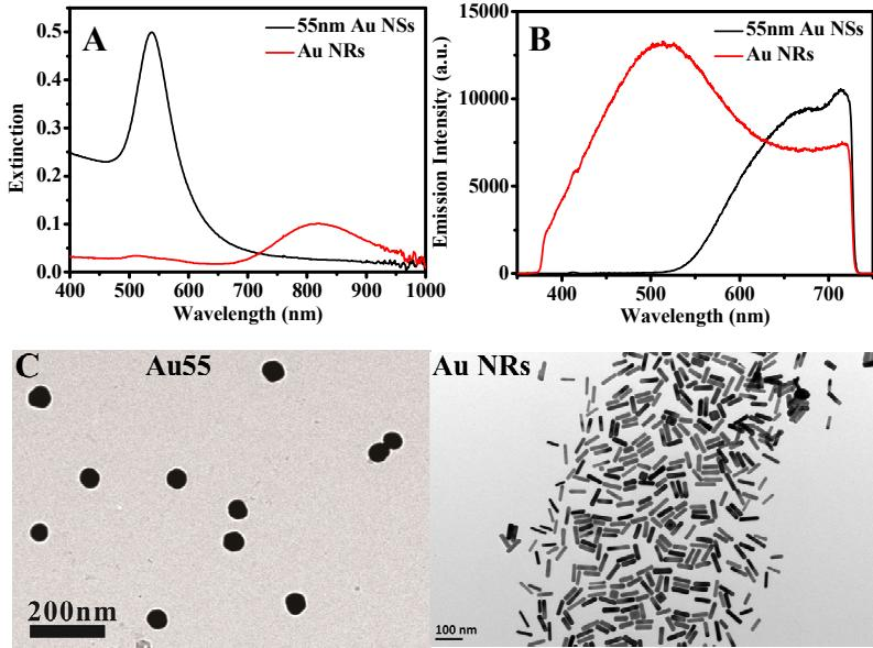
**Figure S6.** (a) UV-Vis extinction spectra, (b) TPPL spectra of 14.5 pM 55nm Au NSs and 20.4 pM Au NRs (average aspect ratio of 4); (c) TEM images of 55nm Au NSs and Au NRs
