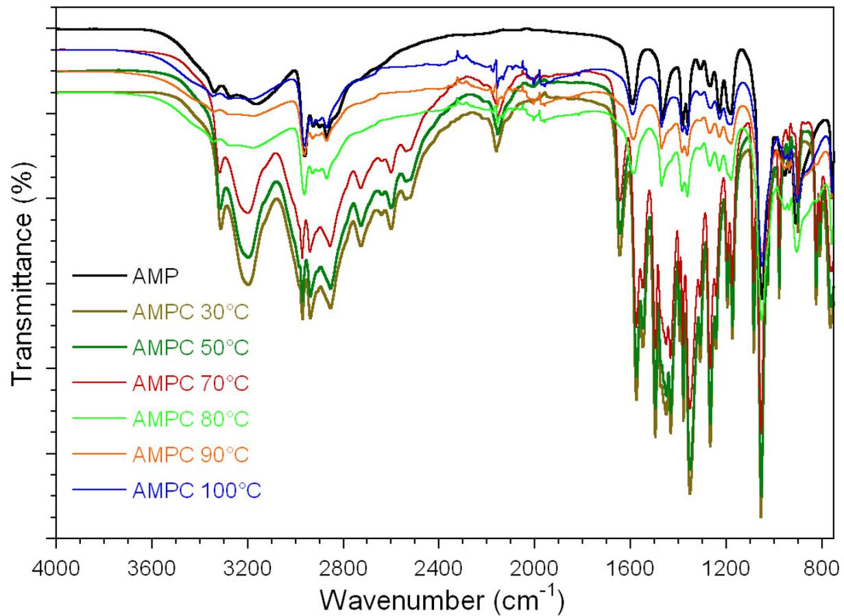
**Figure S4.** FTIR spectrum of AMP-carbamate in the temperature range of 30-100 °C (regenerated AMP appeared in spectra taken at 80 °C and above).
