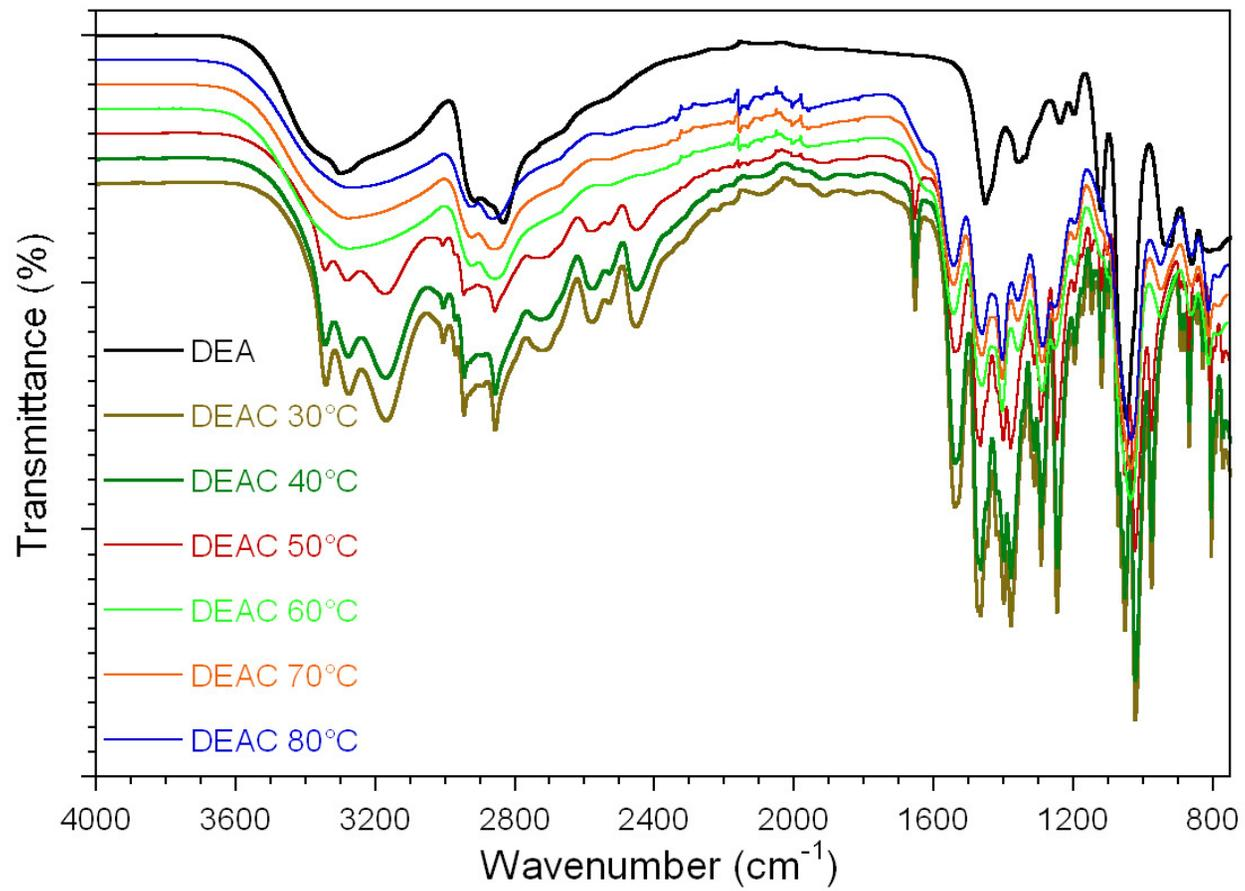
**Figure S5.** FTIR spectrum of DEA-carbamate in the temperature range of 30-80 °C (regenerated DEA appeared above 50 °C).
