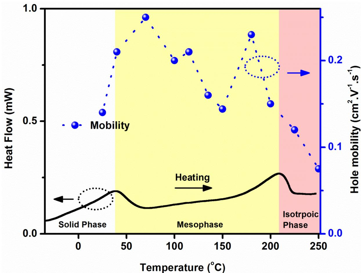
**Figure S18.** Hole mobility of **PBT6** from OFET measurements subjected to annealing in solid phase (room temperature), mesophase (40 °C, 70 °C, 100 °C, 115 °C, 135 °C, 150 °C and 180 °C) and isotropic phase (200 °C, 225 °C and 250 °C). The DSC trace at the bottom indicates the temperature of thermal transition.
