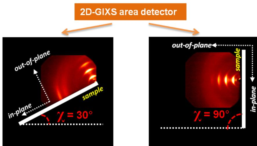
The scheme of sample tilting method under 2D-GIXS
