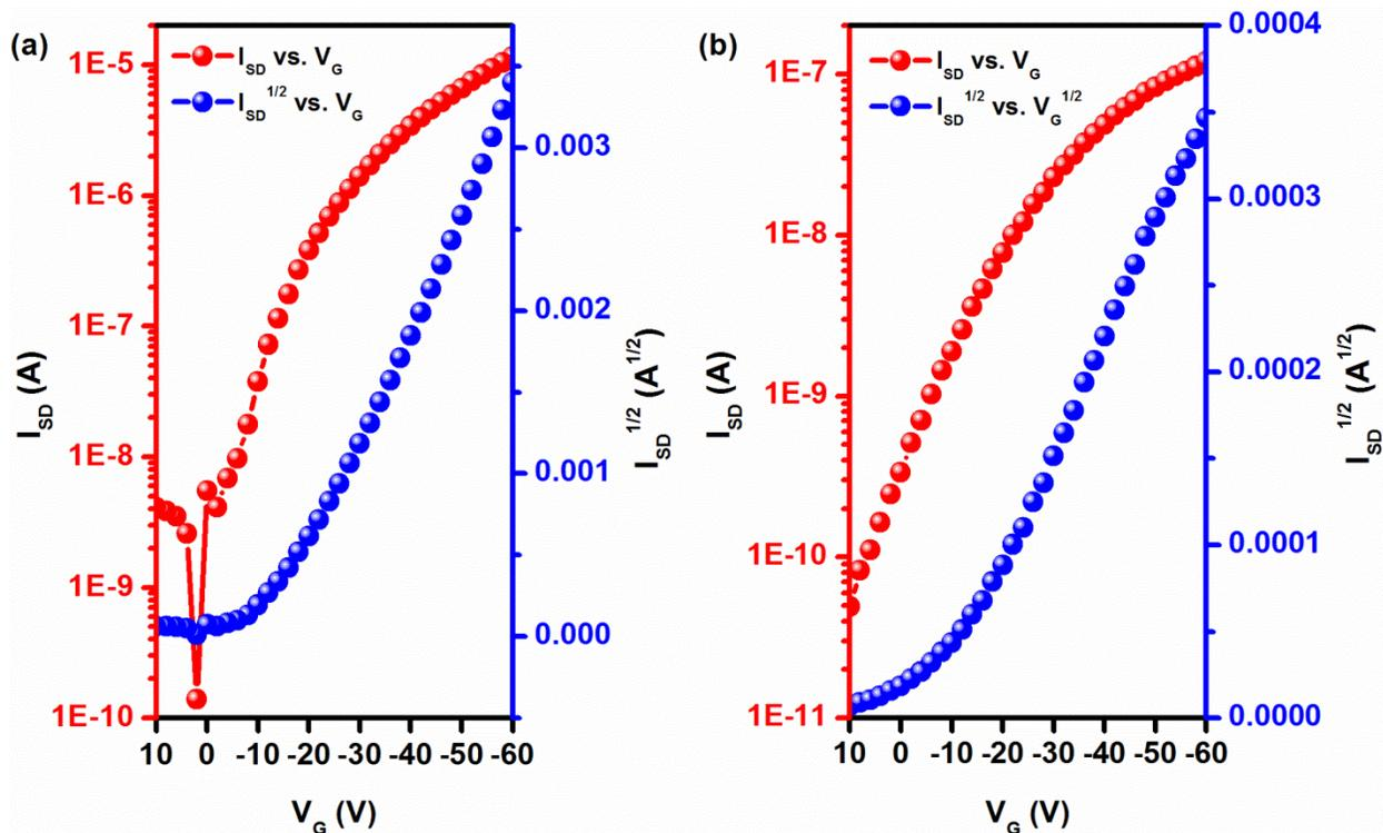
**Figure S16.** Transfer characterization of OFETs ( $V_{SD} = -80$  V, channel size:  $50 \mu\text{m}$  long x  $2$  mm wide): (a) spin-coated **PBT6(L)** film, and (b) spin-coated **PBT6V2** film.
