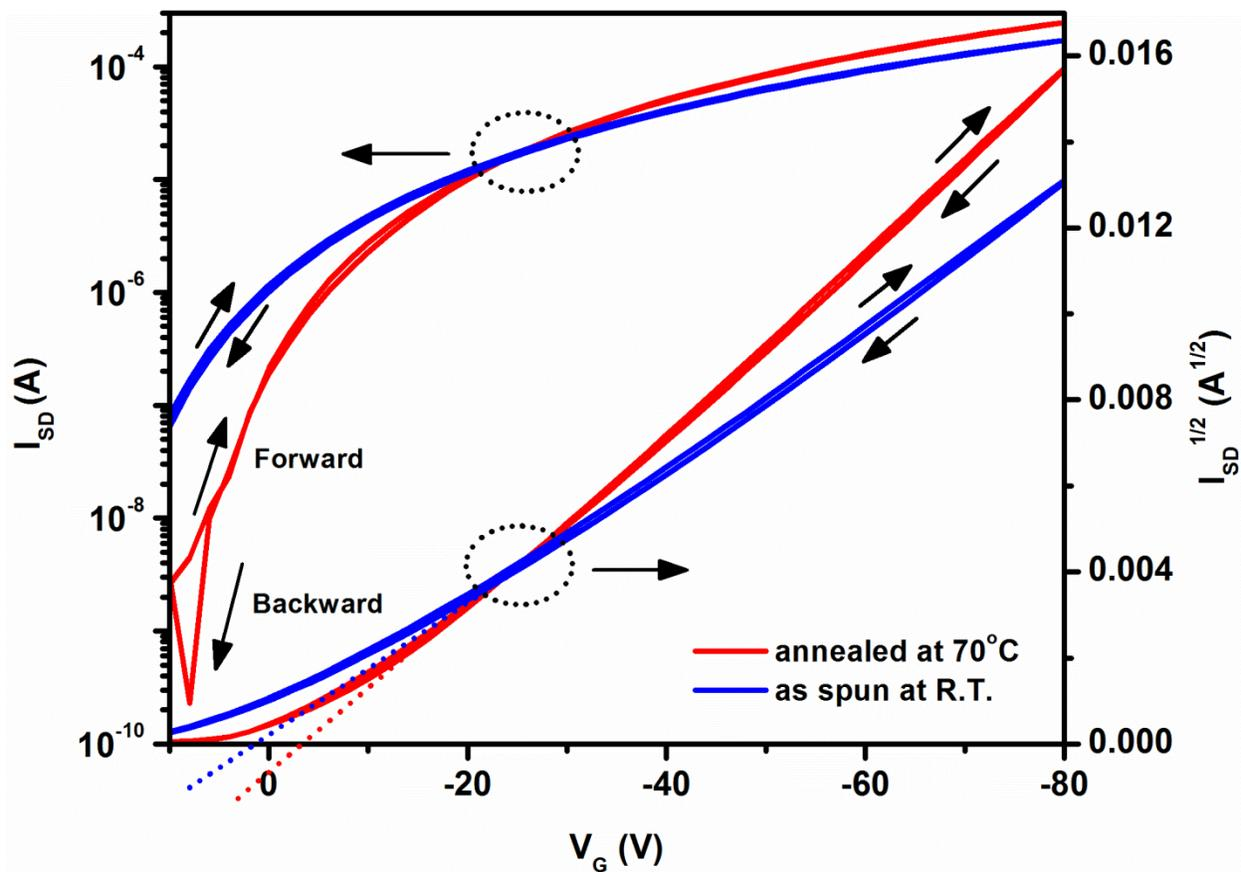
**Figure S20.** Transfer characterizations of OFETs at  $V_{SD} = -80$  V (channel size:  $50 \mu\text{m}$  long x 2 mm wide) based on a spin-coated **PBT6** film as spun at room temperature and annealed at  $70^\circ\text{C}$  for 2 h, in sweeping mode. Arrows signify the sweeping directions (forward: 10 to  $-80$  V; backward:  $-80$  to 10 V) of gate voltage,  $V_G$ .
