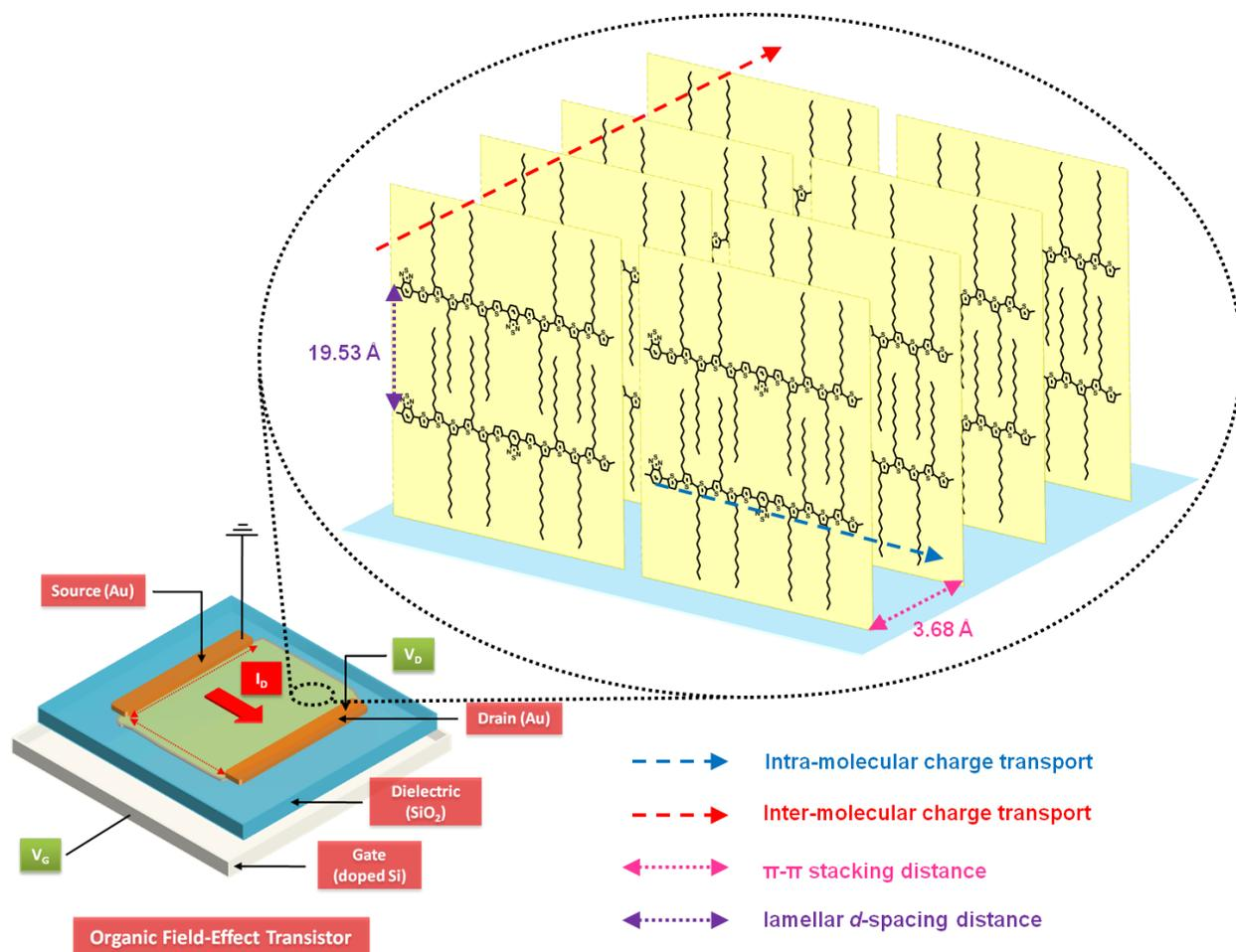
**Figure S15.** Idealized, lamellar  $\pi$  stacking edge-on orientation of **PBT6** thin film onto the bottom contact, bottom gate OFET substrate.
