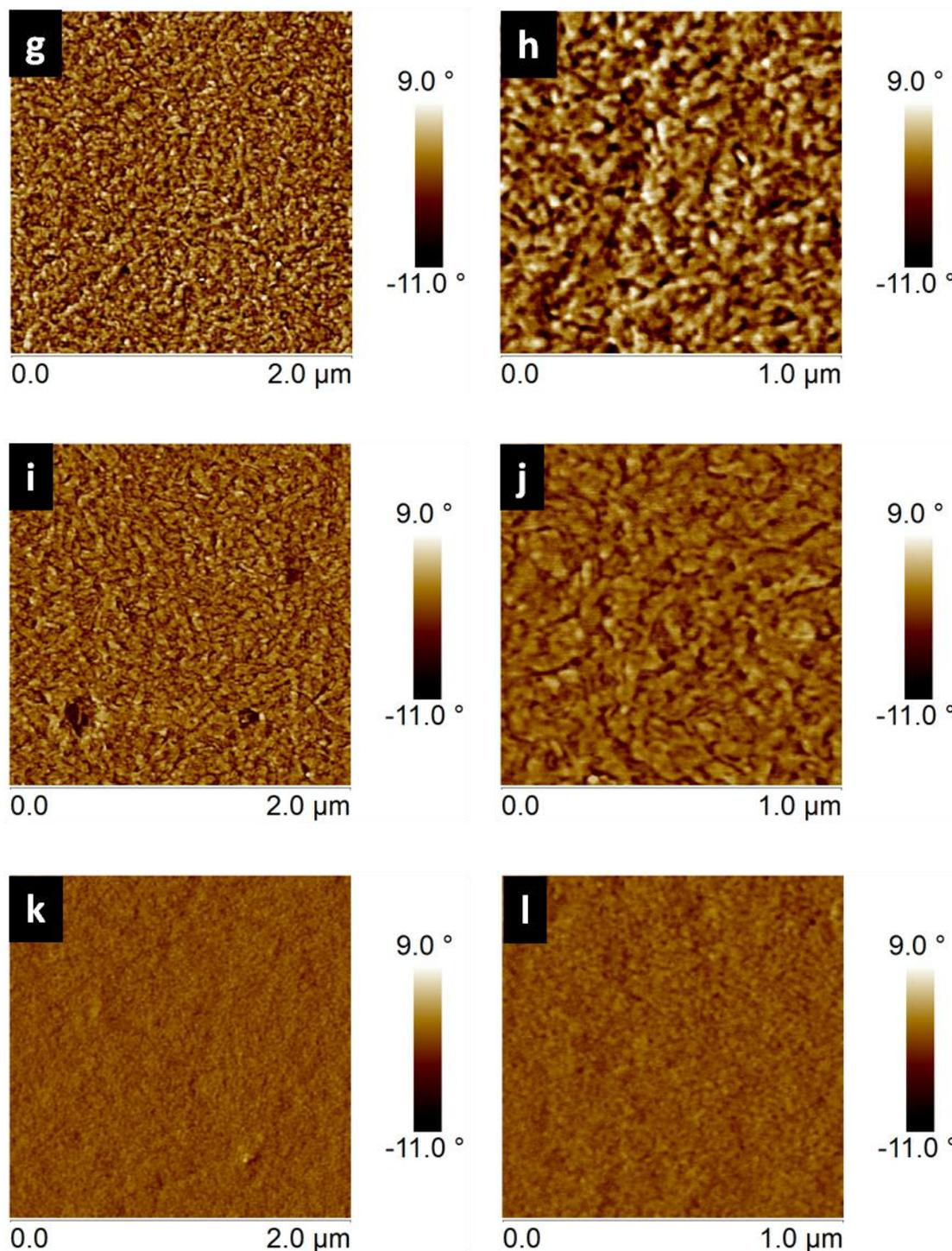
**Figure S19.** Tapping mode AFM phase images of **PBT6** films prepared by spin-coating 8 mg/mL polymer solutions in DCB onto OTS-18 pre-treated OFETs: (a, b) as spun, (c,
