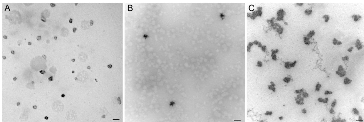
**Figure S1.** TEM images of polydisulfide DNCs. TEM images were acquired for polydisulfide DNCs with hydrodynamic diameters of (A) 59 nm, (B) 91 nm, and (C) 142 nm. The physical sizes measured by TEM, for these three DNC formulations, are  $52\pm 17$  nm,  $86\pm 21$  nm, and  $121\pm 10$  nm, respectively. All scale bars are 100 nm. The grayish shapes are salt crystals due to PBS stock solution.
