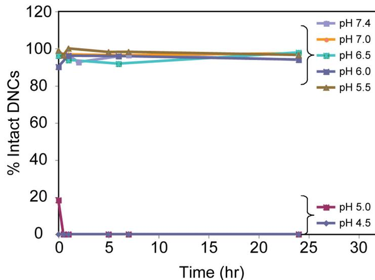
**Figure S3.** Stability of polydisulfide DNCs at various pH as a function of time. Polydisulfide DNCs (59 nm) were added in buffered solutions at various pH and the hydrodynamic diameter was measured over the course of 24 hours, by DLS.
