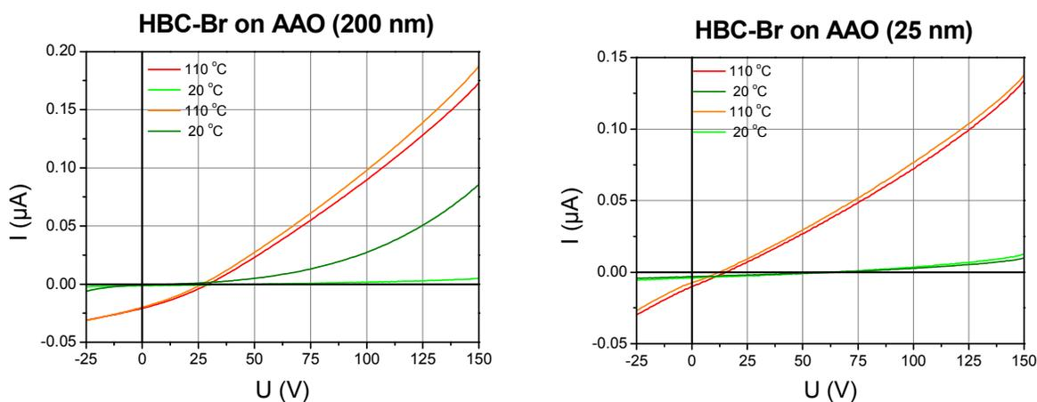
**Figure S5.** I-V characteristics for HBC-Br located inside self-ordered AAO with pore diameters of 200 nm (left) and 25 nm (right) shown at two temperatures.
