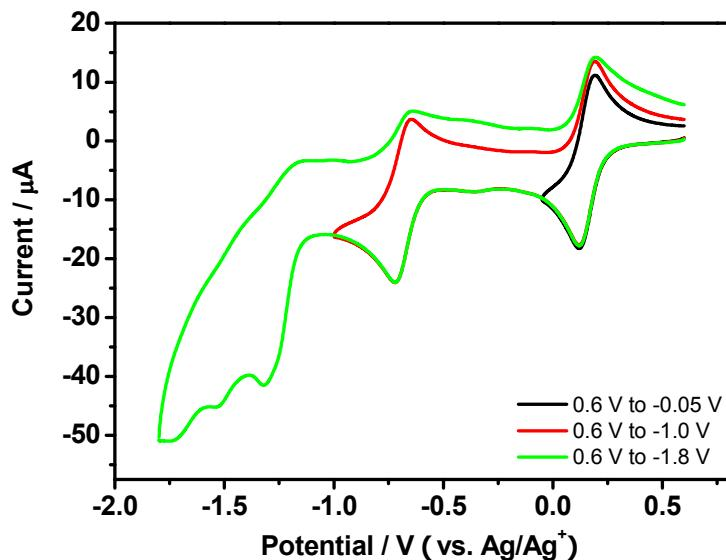
**Figure S1.** Cyclic voltammograms for reductions of 1 mM (n-Bu<sub>4</sub>N)<sub>3</sub>[SVMo<sub>11</sub>O<sub>40</sub>] in MeCN (0.1 M (n-Bu<sub>4</sub>N)PF<sub>6</sub>). Electrode: glassy carbon (diameter 3 mm). Scan rate = 0.1 V s<sup>-1</sup>.
