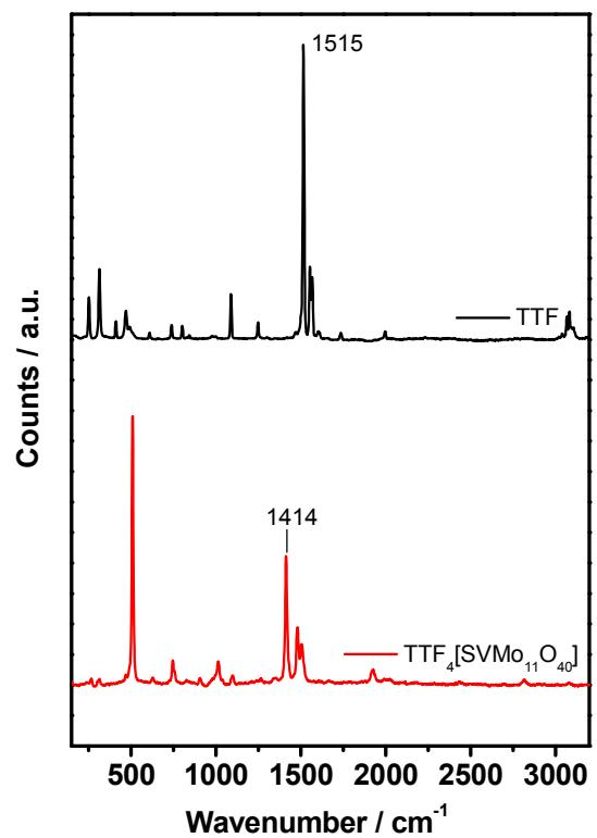
**Figure S2.** Raman spectra for TTF and TTF<sub>4</sub>[SVMo<sub>11</sub>O<sub>40</sub>] solids.
