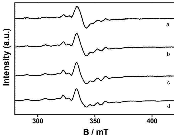
**Figure S3.** EPR spectra of  $\text{TTF}_4[\text{SVMo}_{11}\text{O}_{40}]$  solid (prepared by the solution phase reaction) in the temperature range 290 K to 110 K: (a) 290 K, (b) 210 K, (c) 150 K, (d) 110 K. Spectrometer settings: a) - d) microwave frequency 9.436 GHz; microwave power 0.105 mW; receiver gain  $5.0 \times 10^4$ ; 100 kHz modulation amplitude 1.0 G; scan range/time 1400 G/84 s.; time constant 41s.
