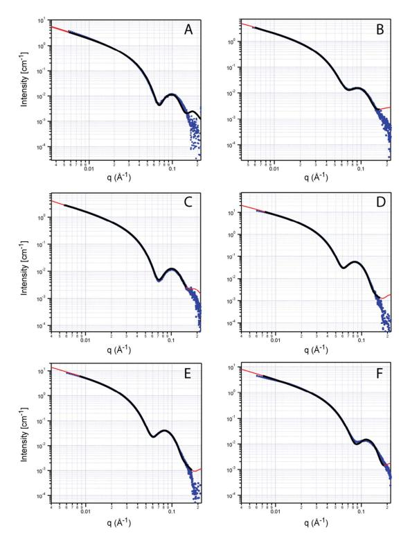
**Figure S2**. SAXS traces and fits of PA **1** (A), PA **2** (B), PA **2** irradiated for 10 min (C), PA **3** (D), PA **4** (E), and PA **5** (F). The blue dots represent the raw data. The solid red line represents the best fit to a core-shell cylinder form factor given by the equations below, where the core was allowed to be polydisperse according to a log-normal distribution. The solid black line represents the portion of the curves where fits were performed.
