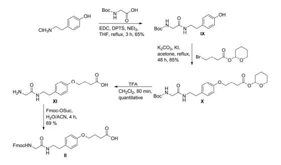
Scheme S2. Synthesis of non-photocleavable Fmoc-amino acid II.
