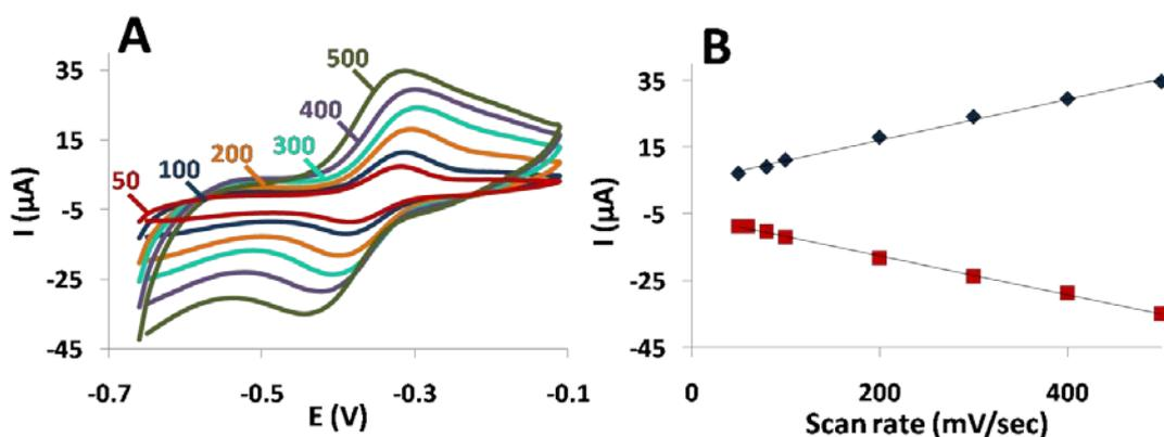
**Figure S7:** (A)-Cyclic voltammograms of a gold disc electrode, modified with **2** under different potential scan rates (in mV/sec) and (B)- Peak current dependence on the potential scan rate, red - cathodic peak current, blue - anodic peak current. Middle point potential is -350 mV vs. Ag/AgCl electrode.
