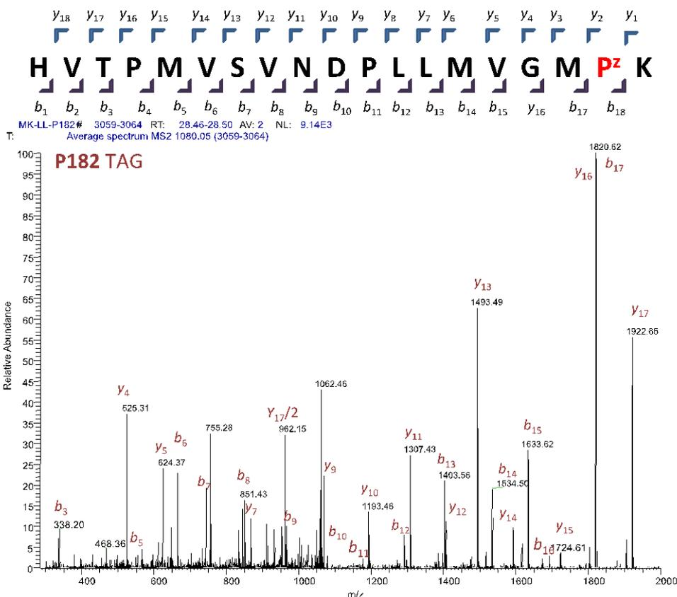
**Figure S6:** MS/MS spectrum of the peptide from P182TAG, containing Az-Phe (labeled as P<sup>z</sup>). The expected fragment ion masses are shown in the spectrum.
