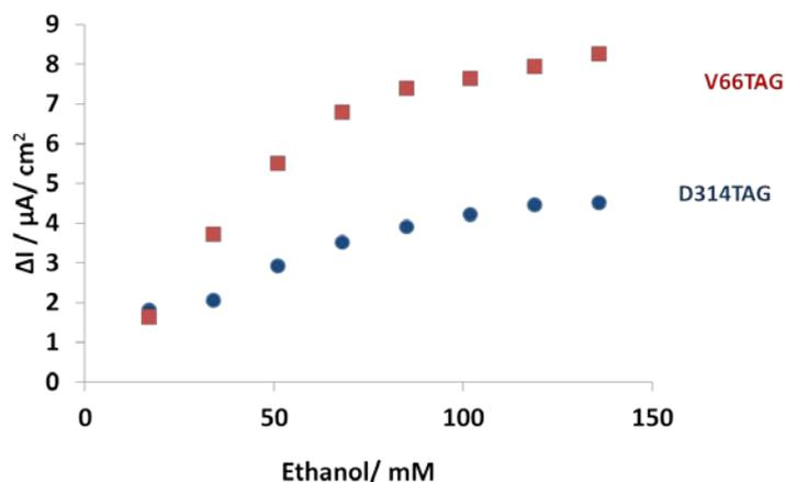
**Figure S8:** Amperometric response of *E. coli* attached to a gold working electrode, upon a 'click' reaction with **2**, under applied potential of  $-0.3\text{V}$  (vs.  $\text{Ag}/\text{AgCl}$ ) to changing ethanol concentrations. (ca.  $150\text{mM}$  equals 1% ethanol in our system).
