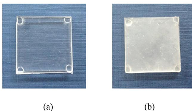
Supplementary Fig. 1. Polydimethylsiloxane (PDMS) chamber for static culture (a) without a Parylene-C coating and (b) with a Parylene-C coating.
