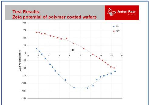
**Figure S1.** The zeta potential of the anionic (AN) and cationic (CAT) polymer brush sample. Note that the isoelectric point (IEP) of the AN sample is estimated at a pH 3.2, while the isoelectric point of the CAT sample is estimated at pH 8.0.
