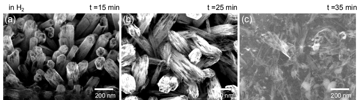
Figure S3. SEM images showing the morphological evolution of the ZnO nanorods after thermal annealing in H 2 ambient at 480 °C for 15 min (a), 25 min (b) and 35 min (c).
