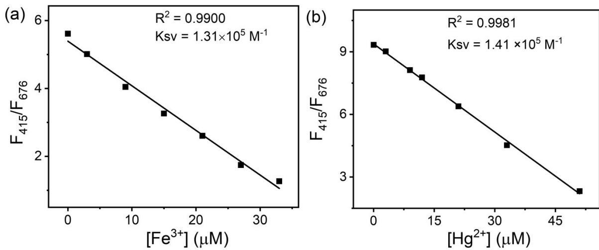
**Figure S10** Stern-Volmer curves of **DPQ-Eu** towards (a)  $\text{Fe}^{3+}$  and (b)  $\text{Hg}^{2+}$ .
