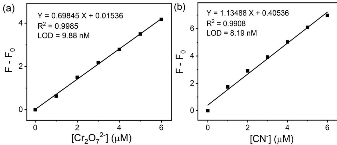
**Figure S17** The detection limits of **DPQ-Eu** towards (a)  $Cr_2O_7^{2-}$  ( $n = 10$ ,  $\sigma = 0.0023$ ) and (b)  $CN^-$  ( $n = 10$ ,  $\sigma = 0.0031$ ) by  $3\sigma/k$  in water, where  $\sigma$  is the standard deviation of blank measurement,  $k$  is the slope,  $\lambda_{ex}$ : 340 nm.
