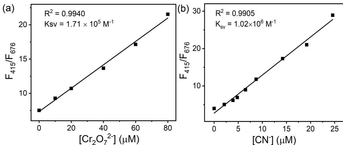
**Figure S16** SV curves of **DPQ-Eu** towards (a)  $\text{Cr}_2\text{O}_7^{2-}$  and (b)  $\text{CN}^-$  anions,  $\lambda_{\text{ex}}$ : 340 nm.
