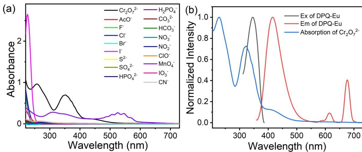
**Figure S23** (a) Absorption spectra of various anions and (b) excitation and emission spectra of **DPQ-Eu** with the absorption of  $\text{Cr}_2\text{O}_7^{2-}$ .
