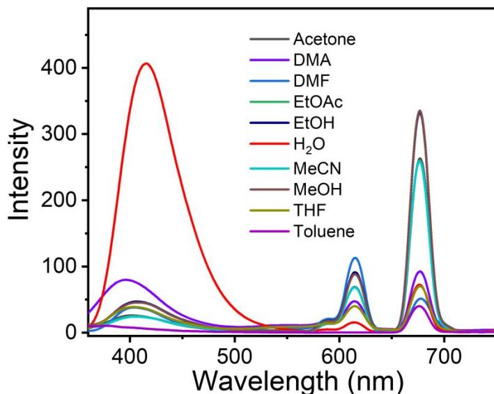
**Figure S8** Emission spectra of **DPQ-Eu** (0.1 mg/3 mL) in different solvents.
