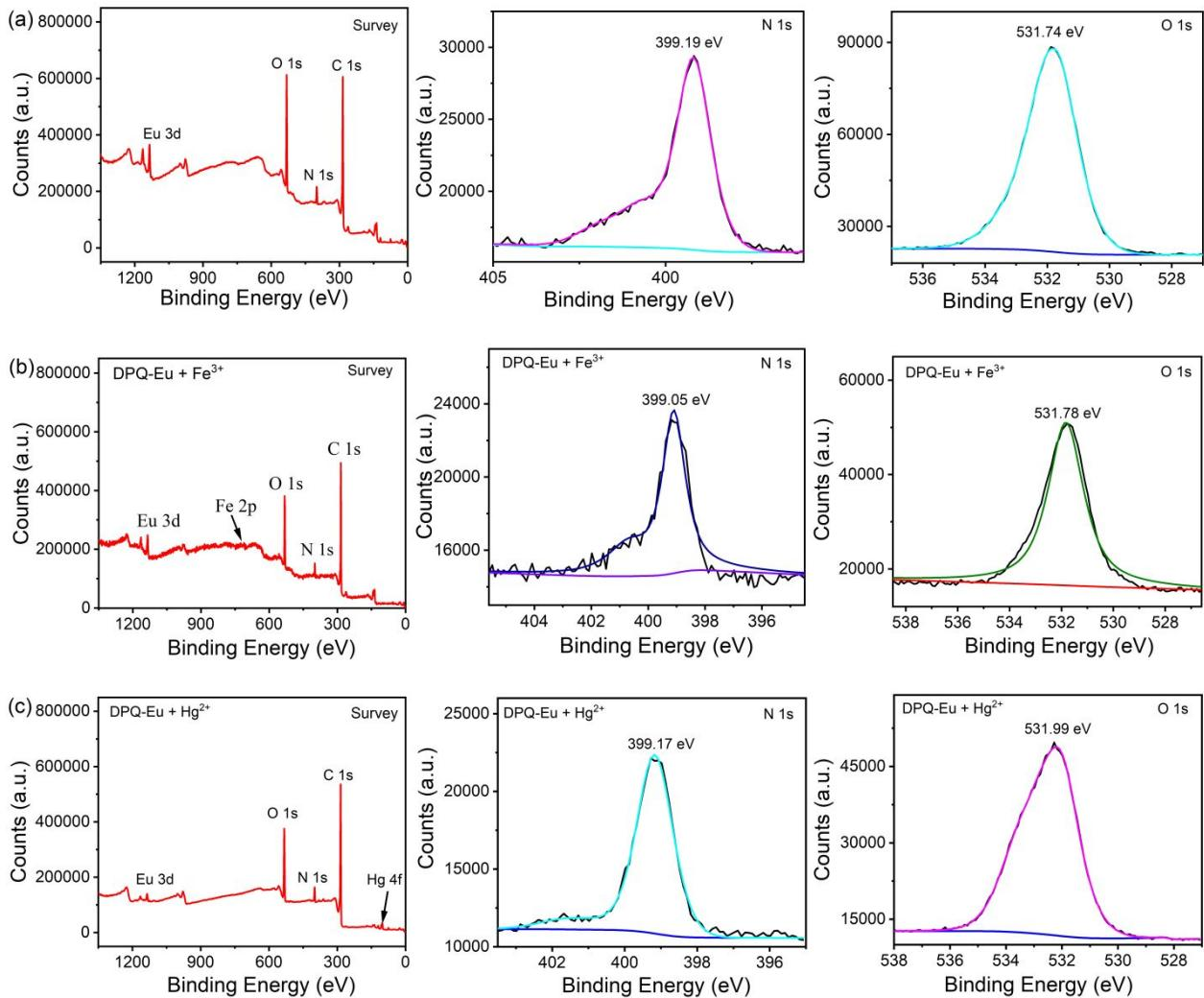
**Figure S22** (a) XPS spectra of **DPQ-Eu**, (b) **DPQ-Eu** treated with  $\text{Fe}^{3+}$ , and (c) **DPQ-Eu** treated with  $\text{Hg}^{2+}$ .
