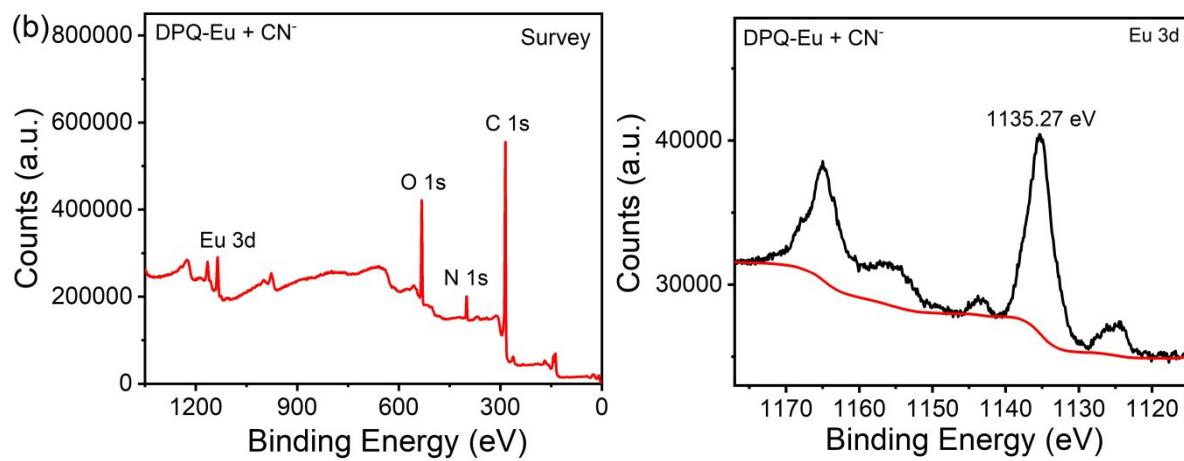
**Figure S25** (a) XPS spectra of **DPQ-Eu**, (b) **DPQ-Eu** treated with  $\text{CN}^-$ . Overall spectra (left), Eu 3d (right).
