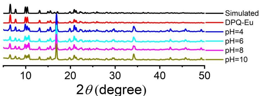
**Figure S3** PXRD patterns for **DPQ-Eu** immersed in water with different pH values for 24 h.
