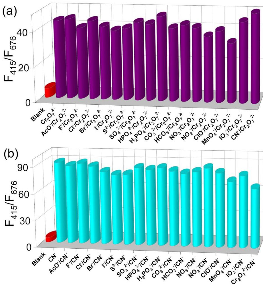
**Figure S20** Emission ratios intensity of the **DPQ-Eu** dispersed in the mixture of other anions and (a)  $\text{Cr}_2\text{O}_7^{2-}$  (190  $\mu\text{M}$ ) / (b)  $\text{CN}^-$  (53.3  $\mu\text{M}$ ),  $\lambda_{\text{ex}}$ : 340 nm.
