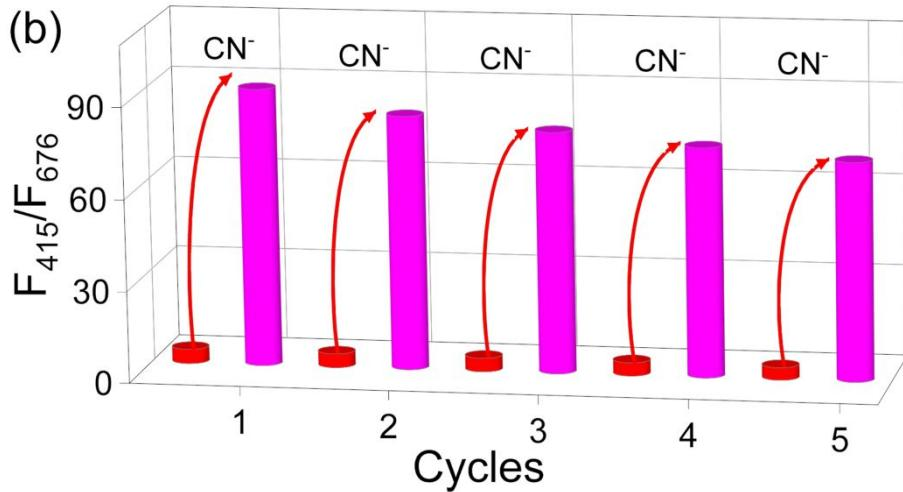
**Figure S19** Recyclable experiments of **DPQ-Eu** for sensing of (a)  $\text{Cr}_2\text{O}_7^{2-}$  (190  $\mu\text{M}$ ) and (b)  $\text{CN}^-$  (53.3  $\mu\text{M}$ ).
