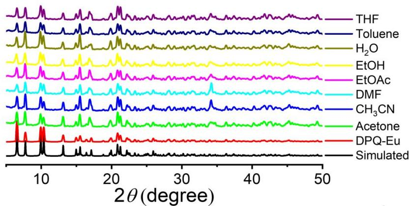
**Figure S2** PXRD patterns for **DPQ-Eu** immersed in commonly used solvents for 24 h.
