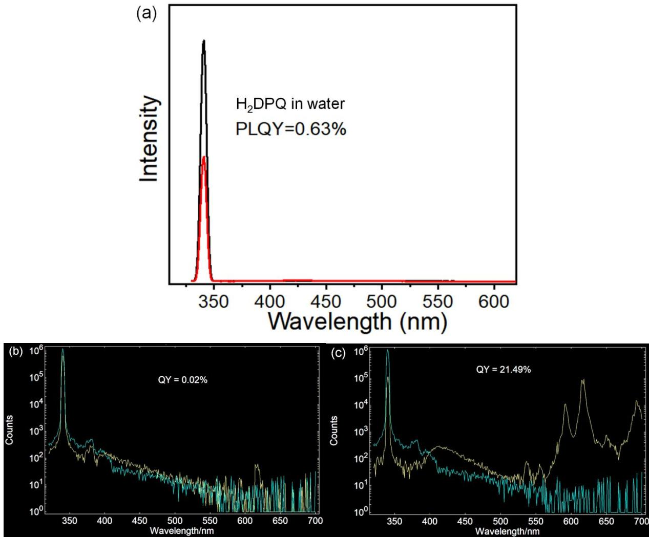
**Figure S6** Absolute quantum efficiency of  $H_2\text{DPQ}$  in (a) water, (b) at solid state, and (c) solid **DPQ-Eu**.
