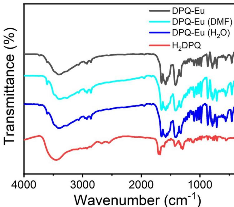
**Figure S1** IR spectra of **H<sub>2</sub>DPQ**, **DPQ-Eu**, and **DPQ-Eu** immersed in H<sub>2</sub>O and DMF for 24 h. (IR (KBr, cm<sup>-1</sup>): **H<sub>2</sub>DPQ**: 3450 (m), 2671 (w), 2549 (w), 1706 (s), 1679 (s), 1606 (w), 1422 (w), 1350 (w), 1313 (w), 1291 (w), 1182 (w), 1128 (w), 1056 (w), 1020 (w), 966 (w), 870 (w), 780 (w), 752 (w), 704 (w); **DPQ-Eu**: 3452 (m), 2929 (w), 1656 (m), 1581 (m), 1417 (s), 1332 (w), 1087 (w), 977 (w), 863 (w), 788 (w), 717 (w).)
