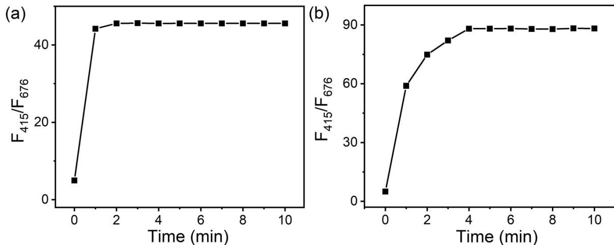
**Figure S18** Emission ratios intensity of **DPQ-Eu** treated by (a)  $Cr_2O_7^{2-}$  ( $190 \mu M$ ) and (b)  $CN^-$  ( $53.3 \mu M$ ) as a function of time,  $\lambda_{ex}$ : 340 nm.
