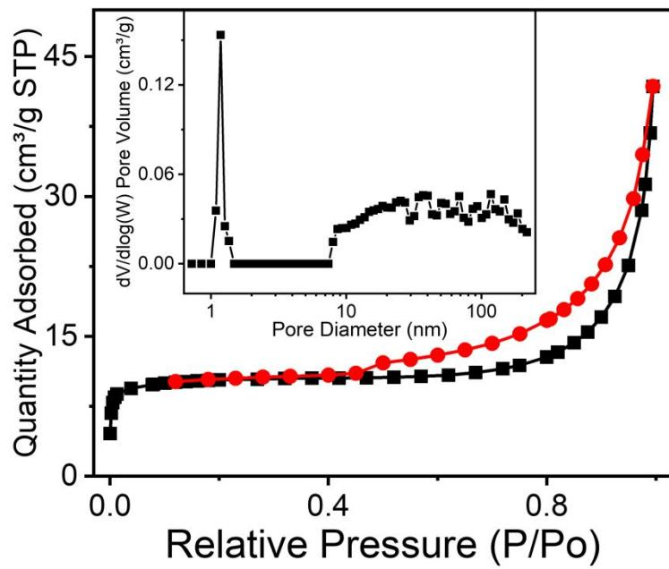
**Figure S5**  $N_2$  adsorption-desorption isotherms of **DPQ-Eu** at 77 K and pore size distribution.
