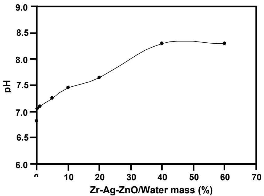
**Figure S8.** Plot of pH versus oxide/water mass percentage
