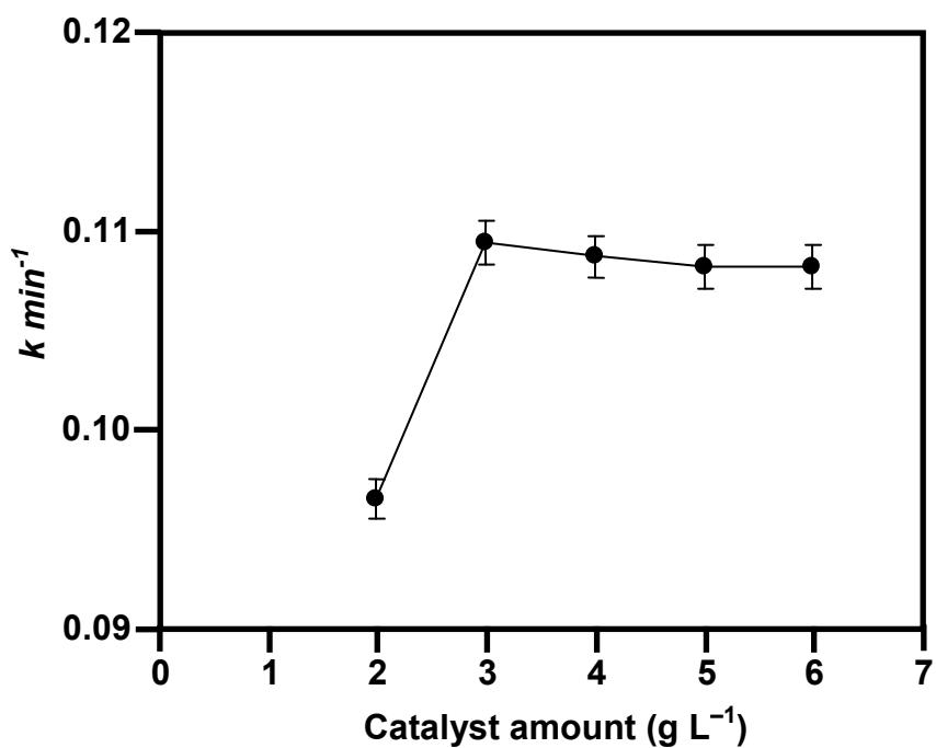
**Figure S9.** Effect of catalyst loading,  $[\text{RR 120}] = 2 \times 10^{-4} \text{ M}$ , Catalyst suspended = 4 wt% Zr-Ag-ZnO, airflow rate =  $8.1 \text{ mLs}^{-1}$ , pH = 7, irradiation time = 20 min;  $I_{\text{solar}} = 1250 \times 100 \pm 100 \text{ lux}$
