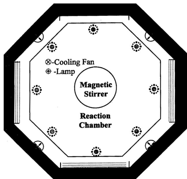
**Figure S2** Schematic diagram of photoreactor.
