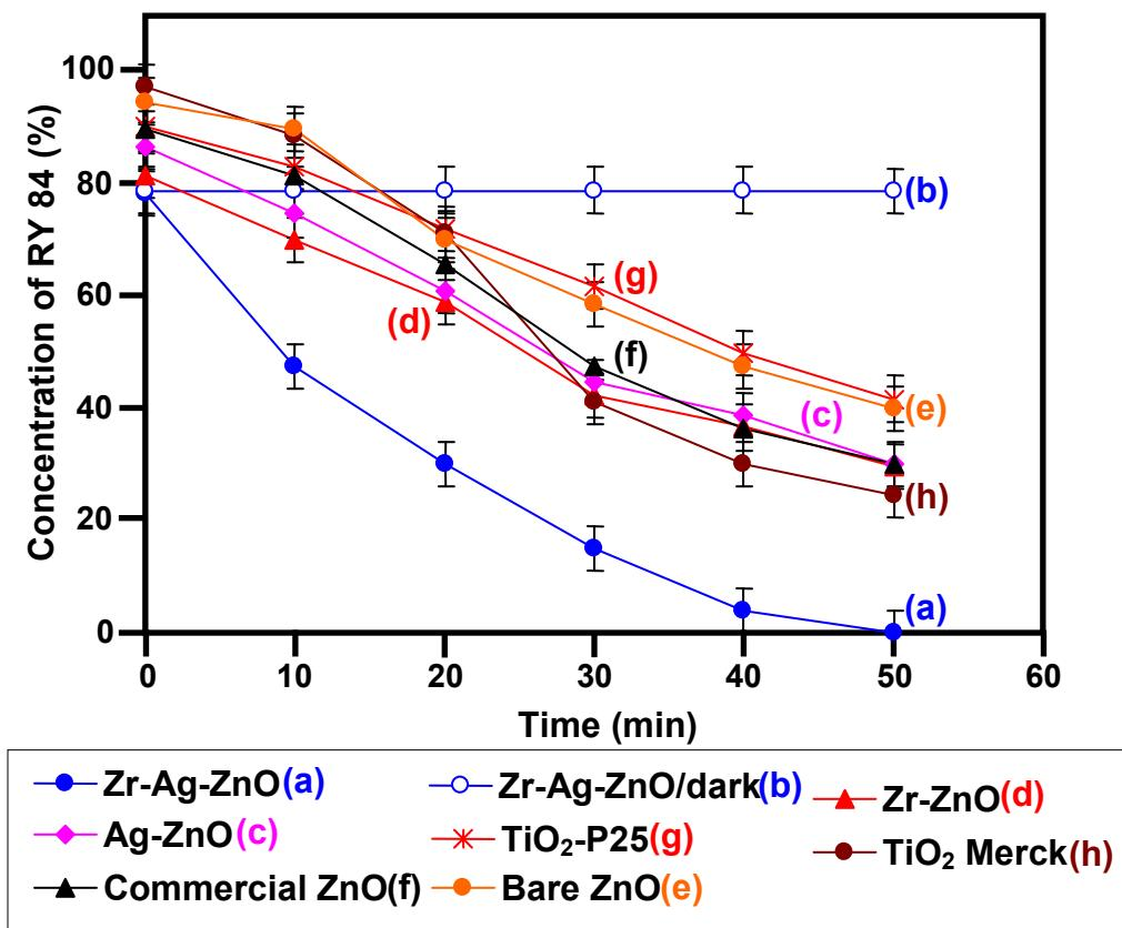
**Figure S6.** Photodegradability of RY 84:  $[RY\ 84] = 5 \times 10^{-4} M$ , catalyst suspended = 3 g pH = 7, airflow rate =  $8.1\ mL\ s^{-1}$ ;  $I_{solar} = 1250 \times 100 \pm 100\ lux$
