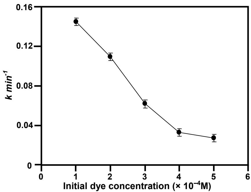
**Figure S10.** Effect of initial dye concentration, pH = 7, 4 wt% Zr-Ag -ZnO suspended = 3 g L<sup>-1</sup>, airflow rate = 8.1 mL s<sup>-1</sup>, irradiation time = 20 min;  $I_{solar} = 1250 \times 100 \pm 100$  lux
