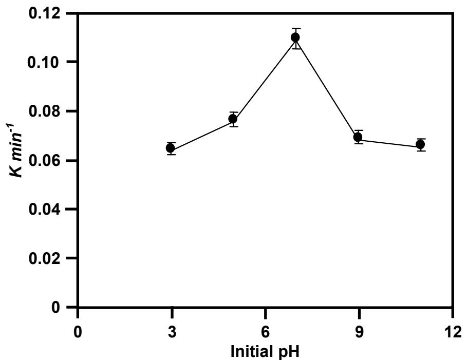
**Figure S7.** Effect of solution pH,  $[\text{RR 120}] = 2 \times 10^{-4} \text{ M}$ , 4 wt% Zr-Ag -ZnO suspended =  $3 \text{ g L}^{-1}$ , airflow rate =  $8.1 \text{ mL s}^{-1}$ , irradiation time = 20 min;  $I_{\text{solar}} = 1250 \times 100 \pm 100 \text{ lux}$
