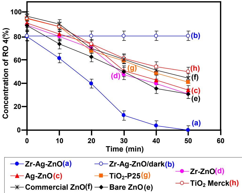
**Figure S4.** Photodegradability of RO 4:  $[RO\ 4] = 5 \times 10^{-4} M$ , catalyst suspended =  $3\ g\ L^{-1}$ , pH = 7, airflow rate =  $8.1\ mL\ s^{-1}$ ;  $I_{solar} = 1250 \times 100 \pm 100\ lux$
