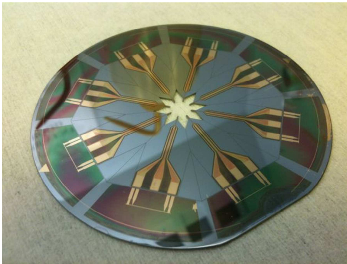
Figure S-1. Patterned sensors on a 3-inch diameter silicon wafer. The laser-trimmed tips and the laser score lines are visible. The wafer thickness is 285 \mu\text{m} .
