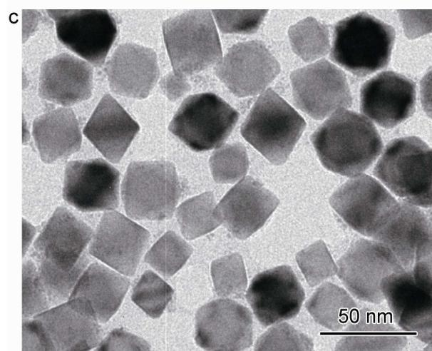
**Supplementary Figure S13.** TEM images of the Pd nanocubes and octahedrons at different sizes used in the investigations: (a) 7-nm nanocubes; (b) 20-nm nanocubes; (c) 21-nm octahedrons.
