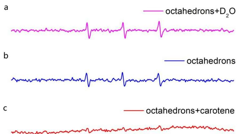
**Supplementary Figure S5.** ESR spectra of the samples after mixing 4-oxo-TMP solution with Pd octahedrons in different conditions: (a) in D<sub>2</sub>O; (b) in H<sub>2</sub>O; (c) in the presence of carotene.
