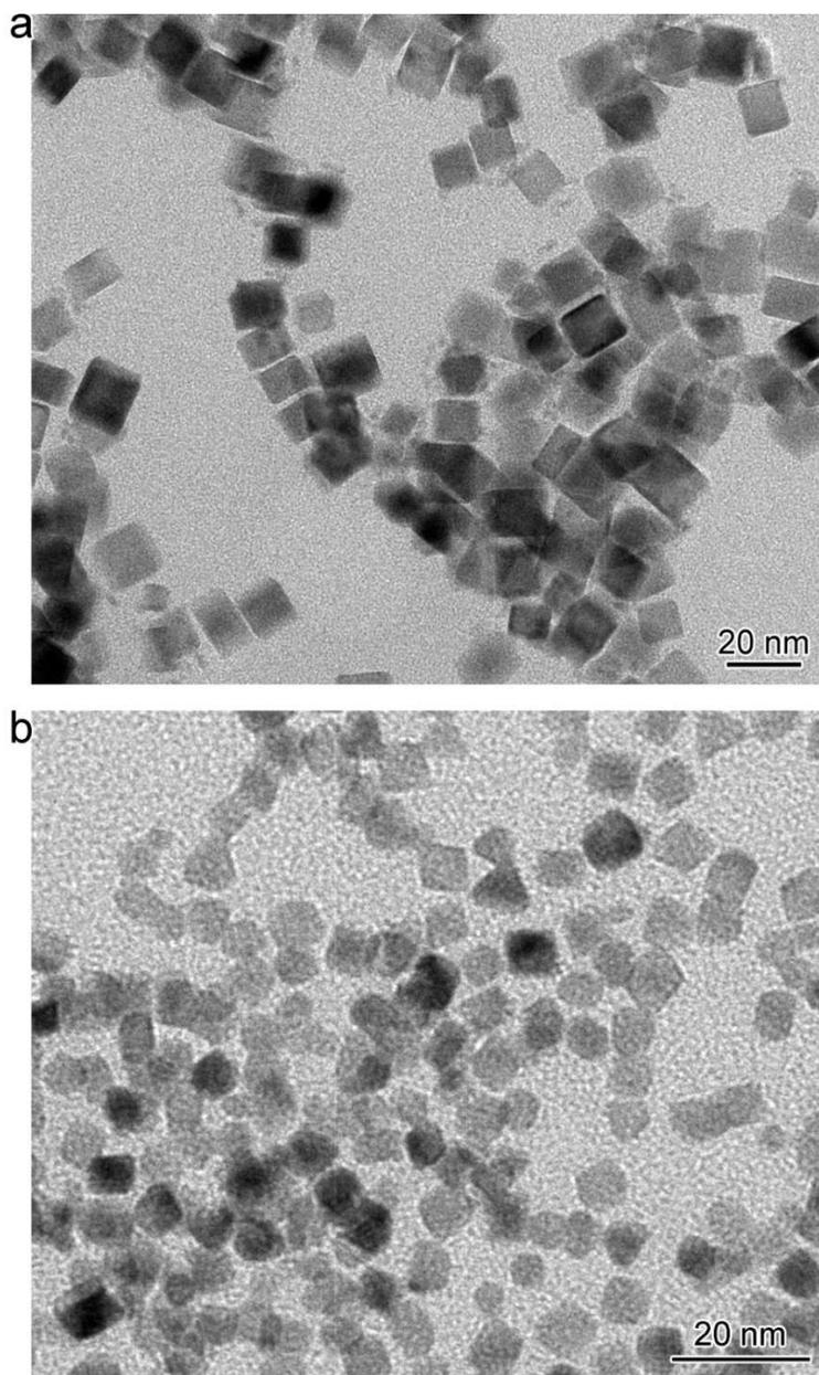
**Supplementary Figure S14.** TEM images of the Pd nanocrystals in Figure 2 after the oxidation of glucose: (a) nanocubes and (b) octahedrons.
