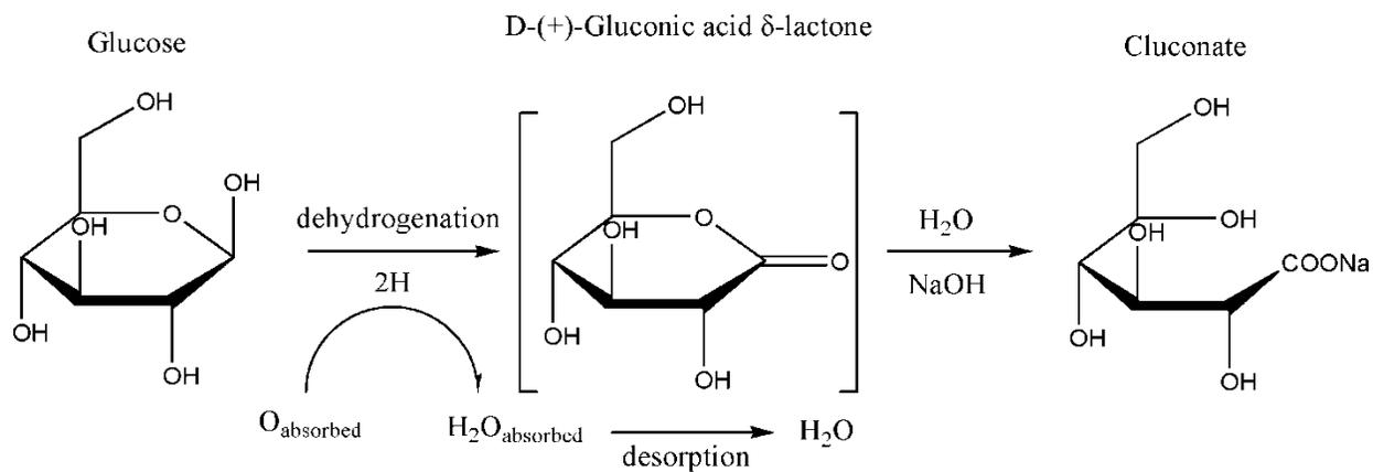
**Supplementary Figure S12.** Reaction pathway for the oxidation of glucose.<sup>5</sup>
