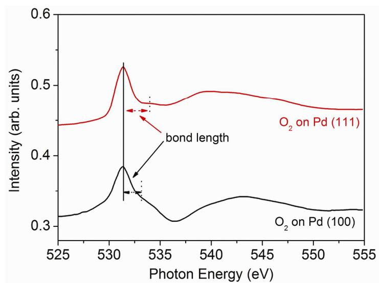
**Supplementary Figure S10.** O *K*-edge NEXAFS spectra of O<sub>2</sub> on Pd nanocubes and Pd octahedrons.
