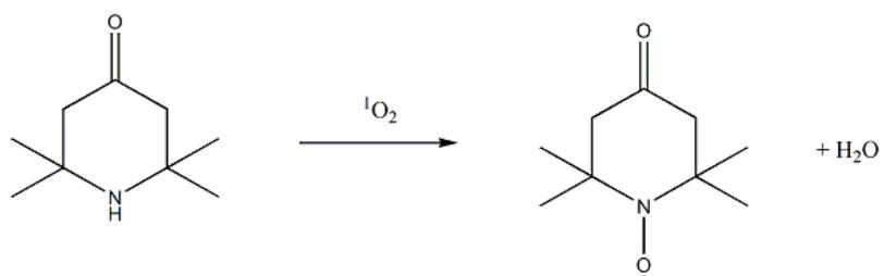
**Supplementary Figure S4.** Reaction pathway for the oxidation of the 2,2,6,6-tetramethyl-4-piperidone (4-oxo-TMP).<sup>4</sup>
