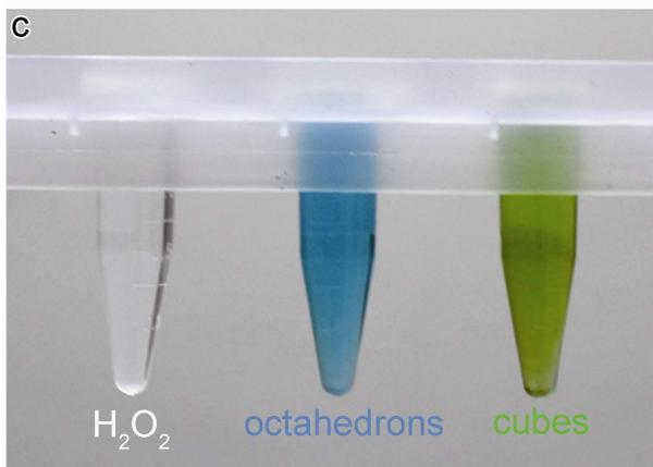
**Supplementary Figure S2.** UV-vis spectra of the samples after mixing TMB solution with different Pd nanocrystals: (a) nanocubes and (b) octahedrons. (c) Photographs of TMB solution mixed with  $H_2O_2$ , Pd octahedrons and nanocubes at 10 °C for 24 h, respectively.
