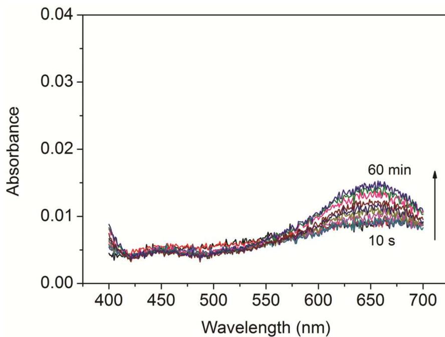
**Supplementary Figure S3.** UV-vis spectra of the samples after mixing TMB solution with hydrogen peroxide.
