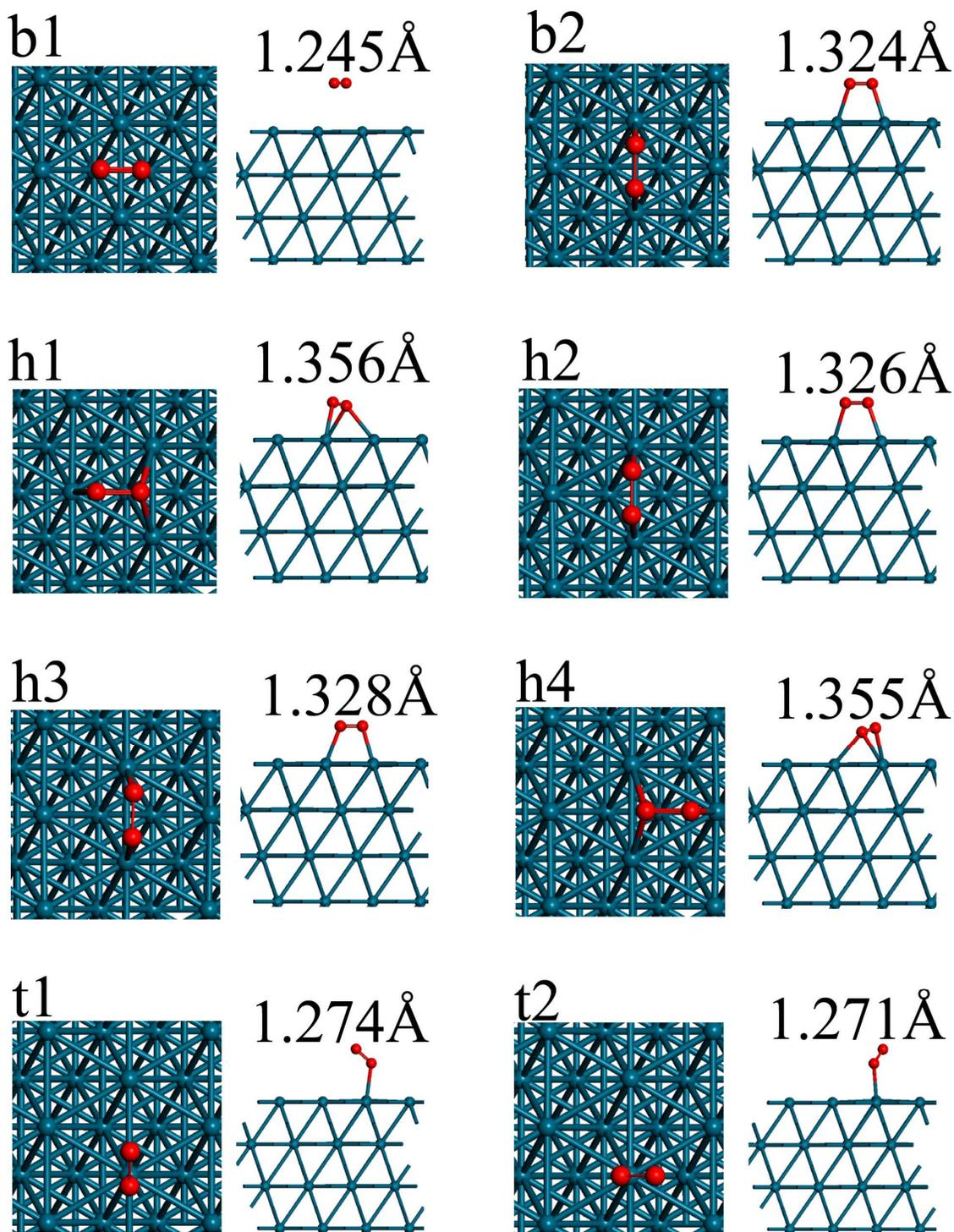
**Supplementary Figure S8.** Eight adsorption configurations of  $O_2$  on Pd(111) facet in the simulation. The spheres in dark cyan color and red color denote the Pd and O atoms, respectively.
