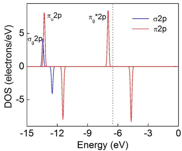
**Supplementary Figure S11.** The projected density of states (PDOS) diagrams of free molecular O<sub>2</sub>.
