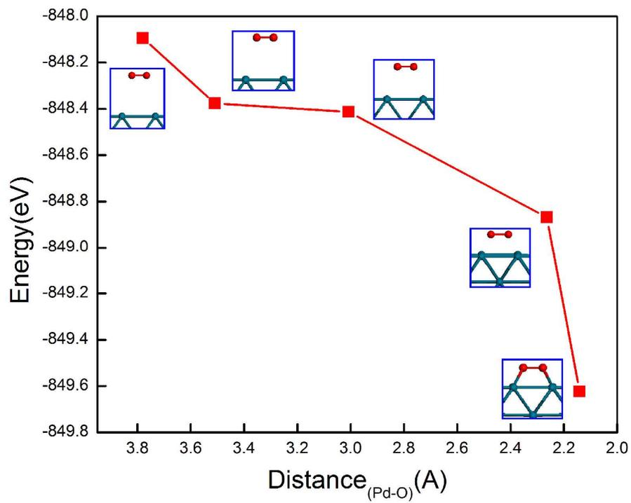
**Supplementary Figure S9.** Curve showing the evolution of the total energy during the adsorption of oxygen to palladium {100} surface.
