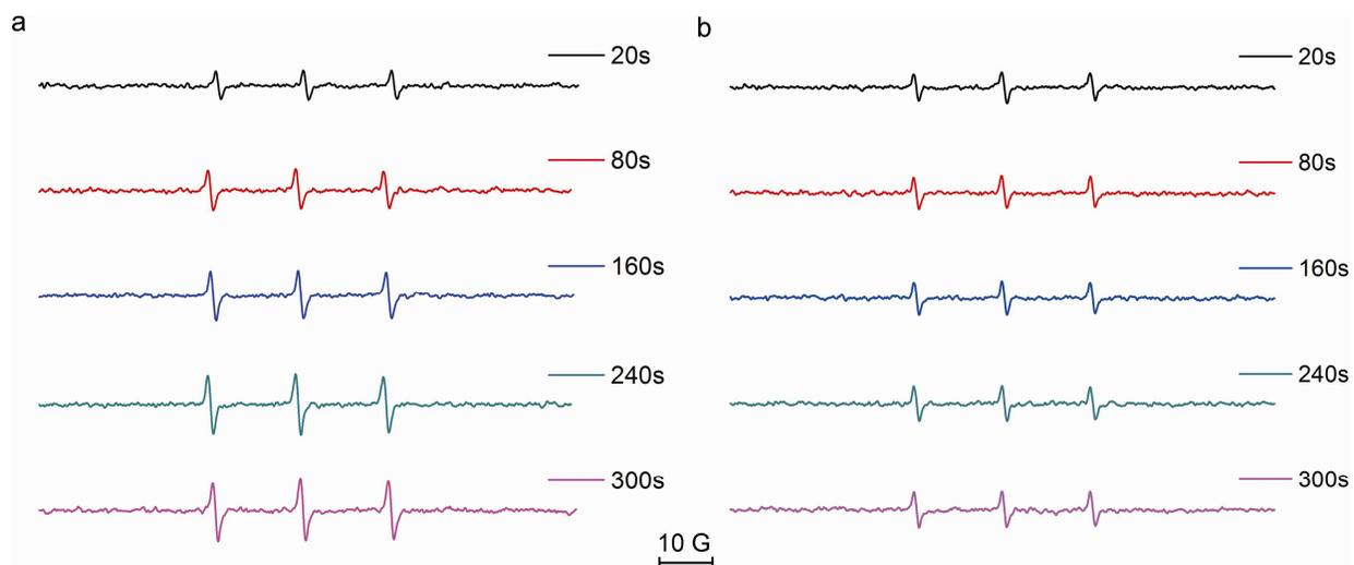
**Supplementary Figure S6.** ESR spectra of the samples after mixing 4-oxo-TMP solution with Pd nanocubes under irradiation of visible light source ( $\nu > 400$  nm) for different time (20-300 sec) in different conditions: (a) without thermostatic adjustment; (b) with thermostatic maintenance at 20°C.
