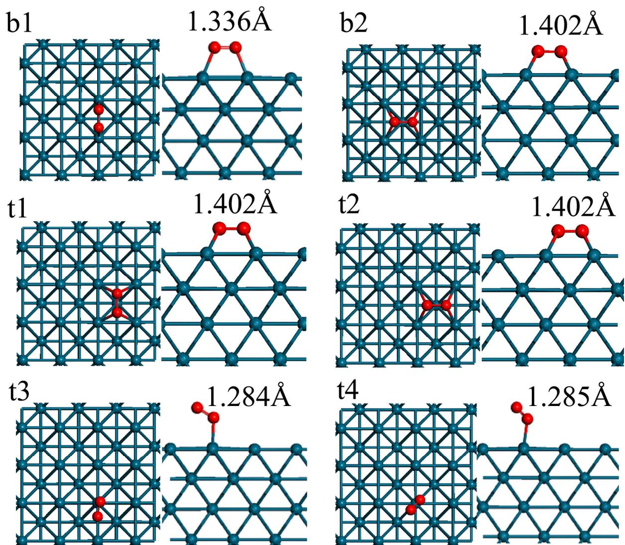
**Supplementary Figure S7.** Six adsorption configurations of  $O_2$  on Pd(100) facet in the simulation. The spheres in dark cyan color and red color denote the Pd and O atoms, respectively.
