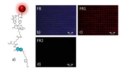
**Figure S3.** a) Molecular structure of immobilized thiol-NTA complexed with His<sub>6</sub>-tagged protein. b-d) Fluorescence images of the surface using different settings:  $\lambda_{exc}$ =350 nm,  $\lambda_{em}$ =420 nm (FB);  $\lambda_{exc}$ =510-550,  $\lambda_{em}$ =590 nm, (FR=FR1);  $\lambda_{exc}$ =650 nm,  $\lambda_{em}$ =670 nm (FR2).
