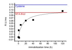
**Figure S7.** Fluorescence intensities of coumarin after immobilization of cysteine<sup>S4</sup> for 1 h (blue line), NTA-thiol for 1 h (red line) and <sup>G174C</sup>TFP (for various time points, squares) through the fluorogenic thio-Michael addition ( $\lambda_{exc}$ =350 nm,  $\lambda_{em}$ =420 nm).
