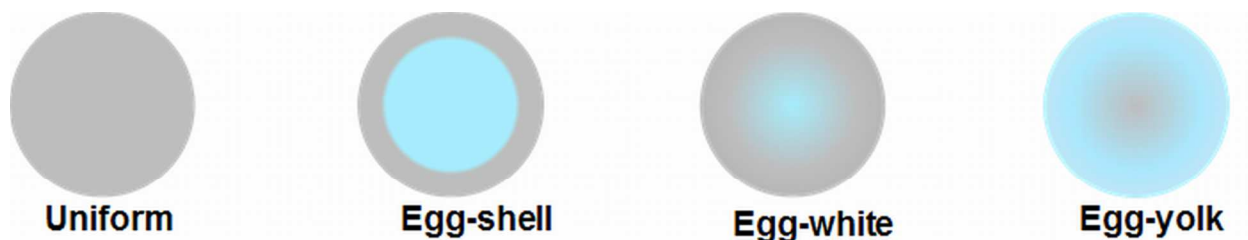
Figure S1. A schematic description of the micro-distributions of an active phase in a cylindrical extrudate as observed when bisected.
