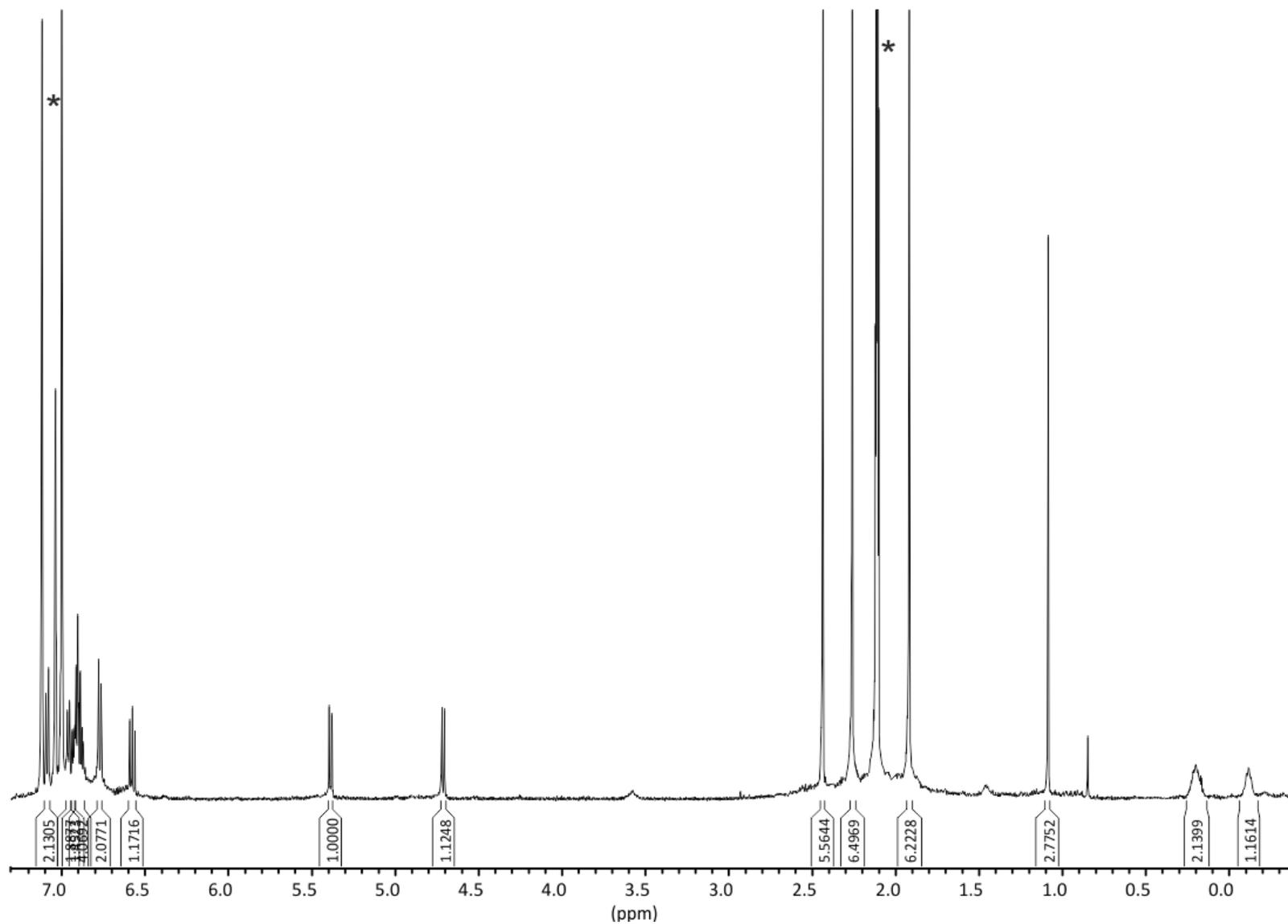
Figure S19. <sup>1</sup>H NMR spectrum (500 MHz, toluene-*d*<sub>8</sub>, 298 K) of the reaction product (6) of 2a' with 1 equiv of NH<sub>3</sub>BH<sub>3</sub>. \* stands for residual solvent signals.
