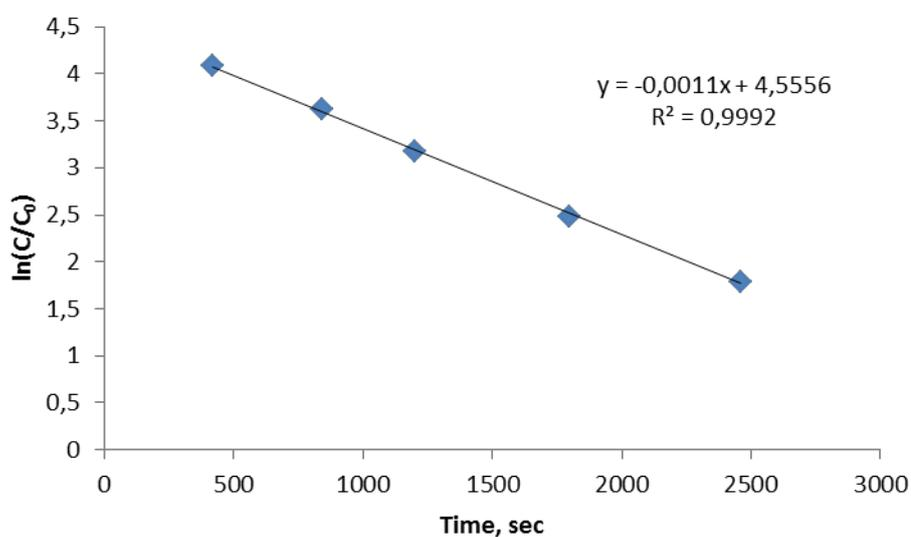
Figure S5. Kinetic data ( $\ln(C/C_0)$  vs. time (s)) for the reaction of alkyl complex 2a' with 1 equiv of  $[\text{Et}_3\text{NH}][\text{BPh}_4]$ , monitored in THF- $d_8$  at  $-10\text{ }^\circ\text{C}$ .
