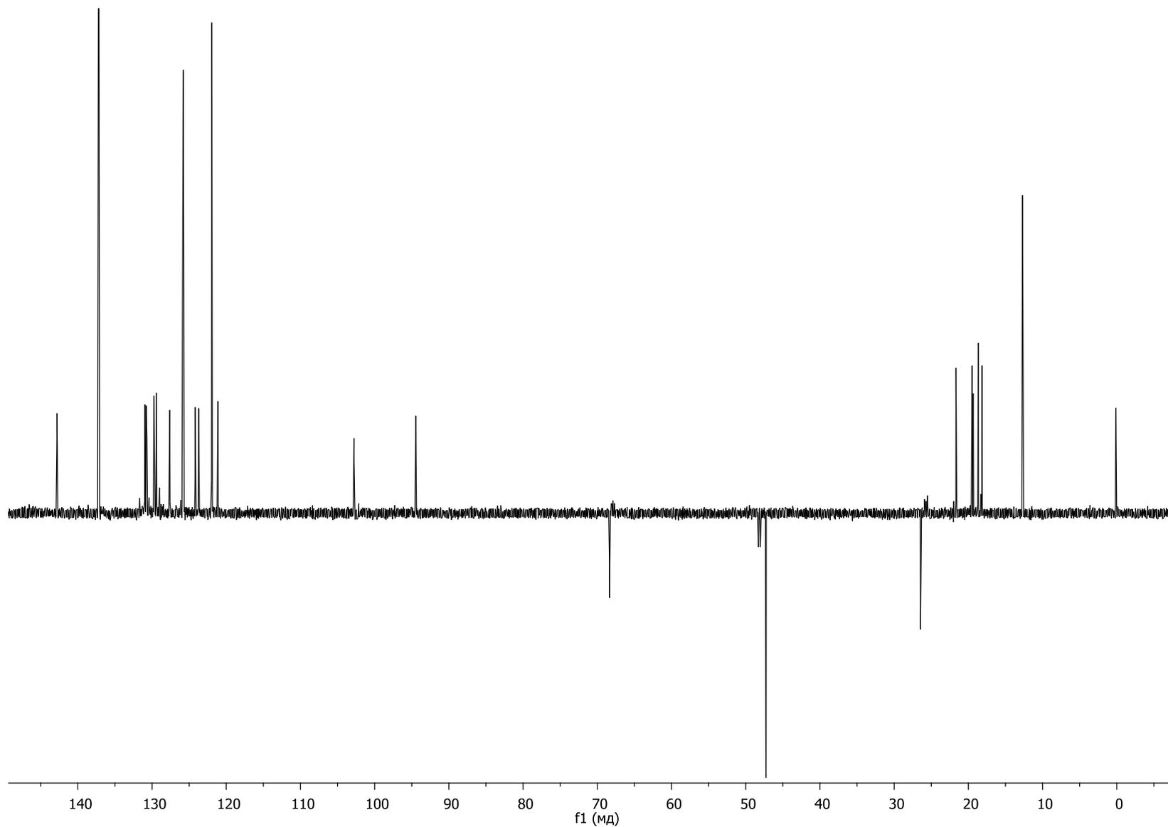
Figure S15.  $^{13}\text{C}$  DEPT 135 NMR spectrum (400 MHz,  $\text{THF-}d_8$ , 273 K) of the reaction product (4) of  $2a'$  with 1 equiv of  $[\text{HNEt}_3][\text{BPh}_4]$ .
