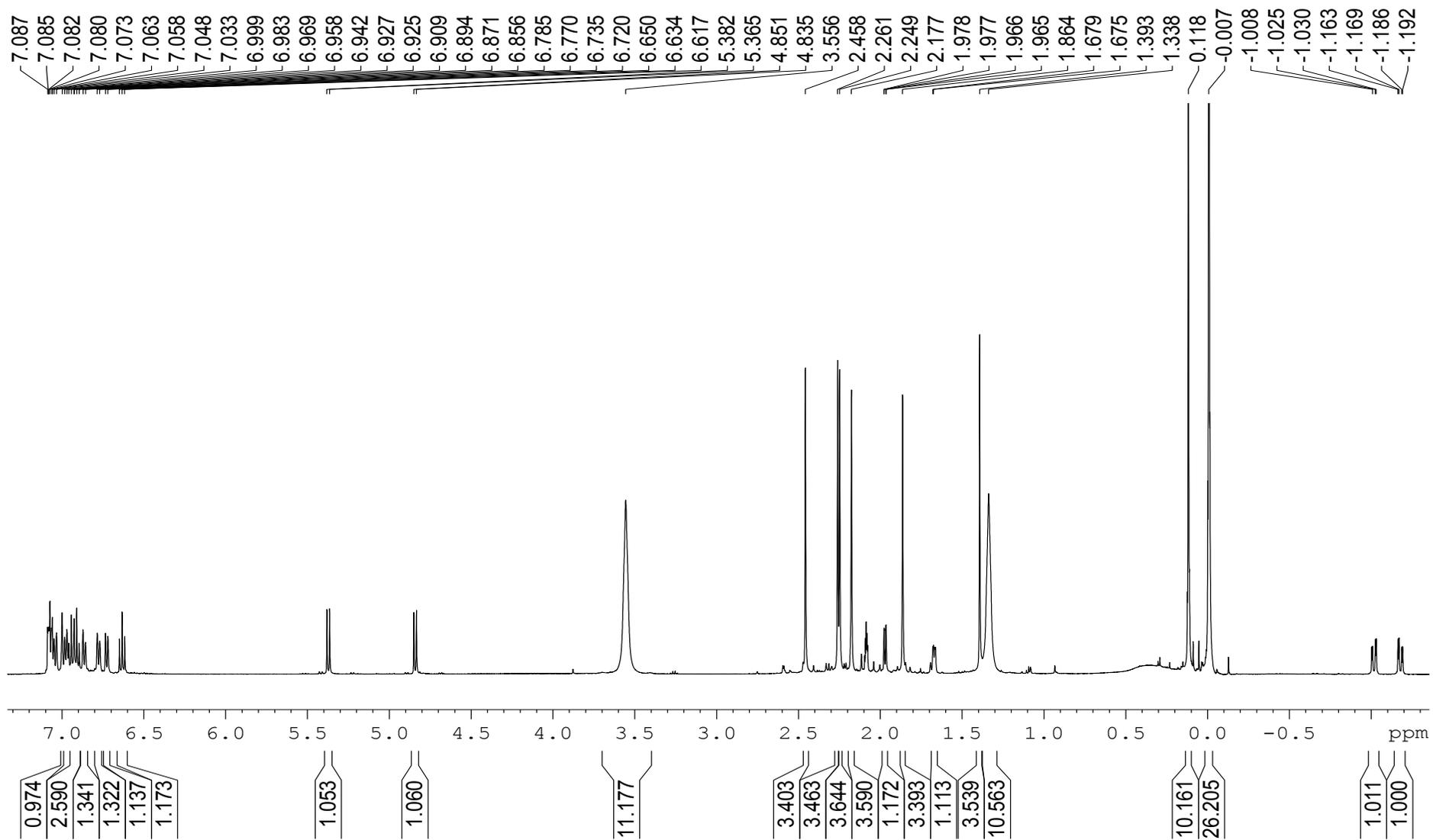
Figure S6.  $^1\text{H}$  NMR spectrum (500 MHz, toluene- $d_8$ , 298 K) of  $\{\text{N}^{\text{Me}_2}\text{NN}^{\text{Me}_2}\text{C}^{\text{Me}}\text{N}^{\text{Me}}-\text{CH}_2\}\text{Y}(\text{CH}_2\text{SiMe}_3)(\text{THF})$  ( $2a'$ ).
