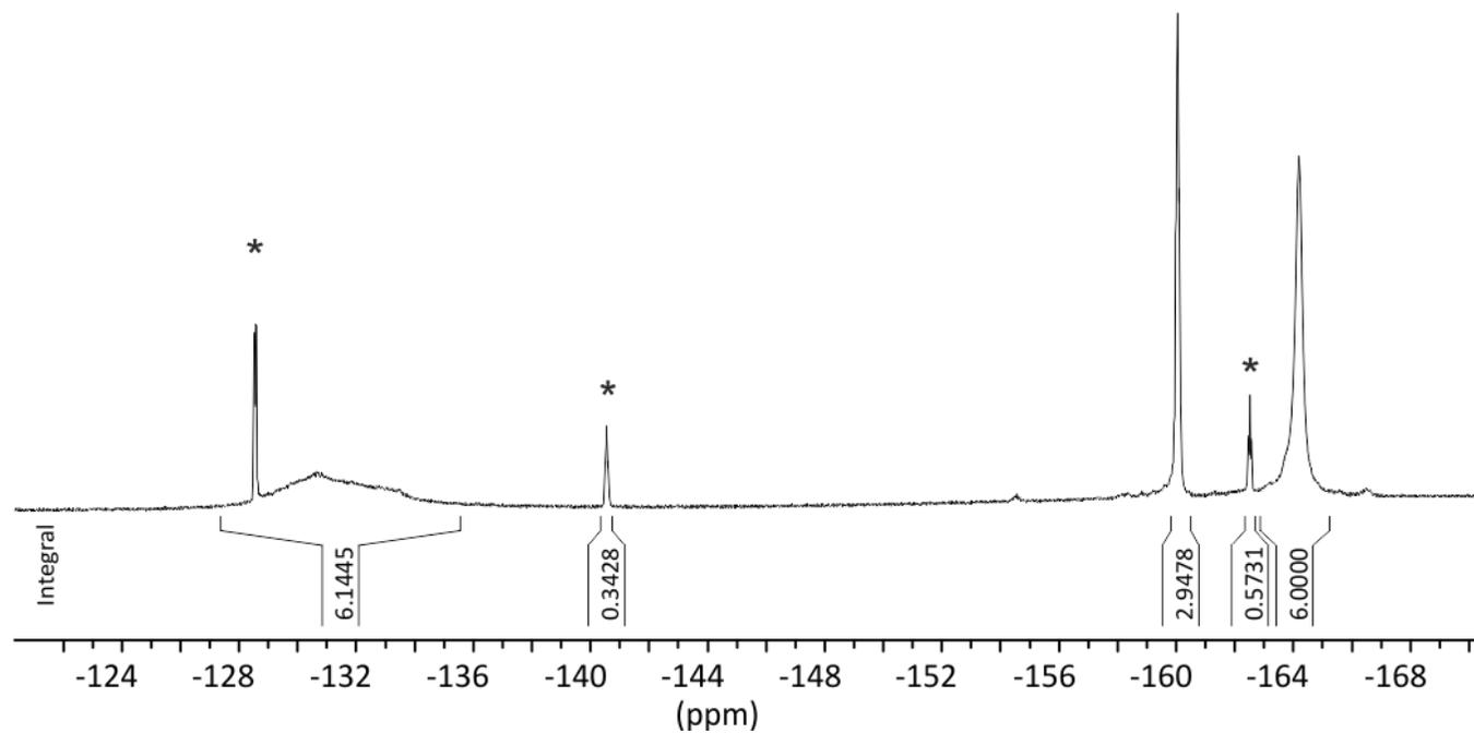
Figure S12.  $^{19}\text{F}\{^1\text{H}\}$  NMR spectrum (376 MHz, toluene- $d_8$ , 233 K) of the reaction product (3) of 2a' with 1 equiv of  $\text{B}(\text{C}_6\text{F}_5)_3$ . \* stand for excess of  $\text{B}(\text{C}_6\text{F}_5)_3$ .
