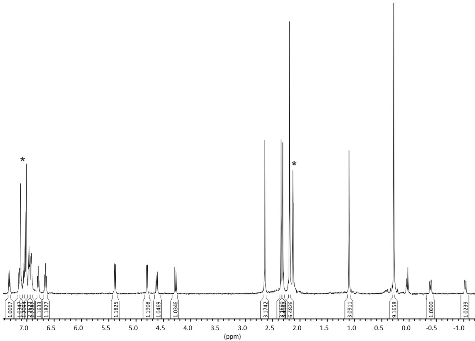
Figure S20.  $^1\text{H}$  NMR spectrum (500 MHz, toluene- $d_8$ , 333 K) of [ $\{\text{N}^{\text{Me}2}\text{NN}^{\text{Me}2}\text{C}^{\text{Me}}\text{N}^{\text{Me}}-\text{CH}_2(\mu\text{-O})\}\text{Y}(\text{CH}_2\text{SiMe}_3)_2$ ] (7). \* stands for residual solvent signals.
