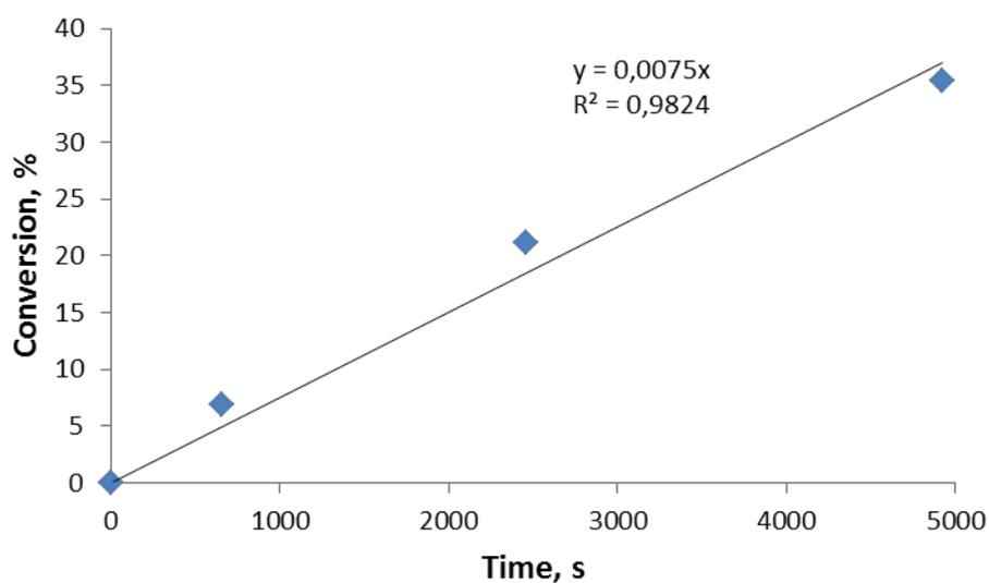
Figure S4. Kinetic data (conversion (%) vs. time (s)) for the intramolecular C–H bond activation reaction in the alkyl complex 2a, monitored in toluene- $d_8$  at  $-30\text{ }^\circ\text{C}$ .
