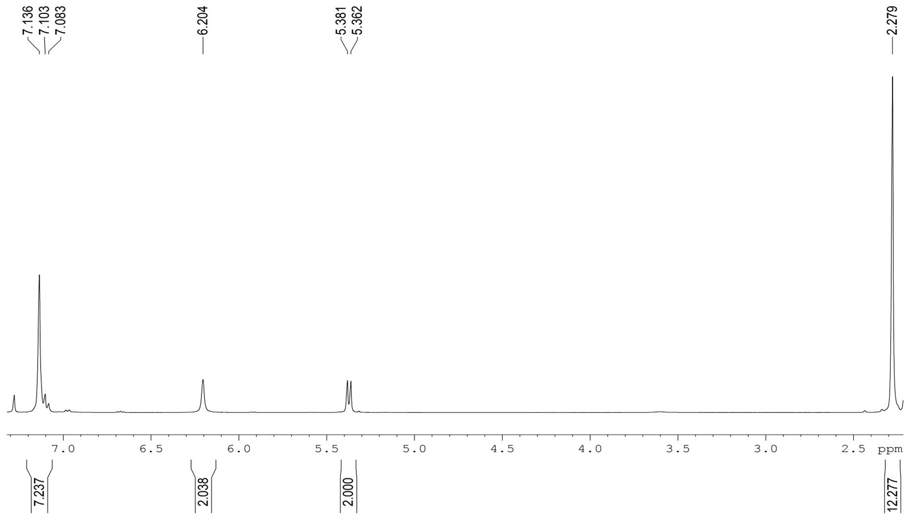
Figure S1. <sup>1</sup>H NMR spectrum (400 MHz, CDCl<sub>3</sub>, 298 K) of (N<sup>Me</sup><sub>2</sub>NN<sup>Me</sup><sub>2</sub>)H<sub>2</sub>.
