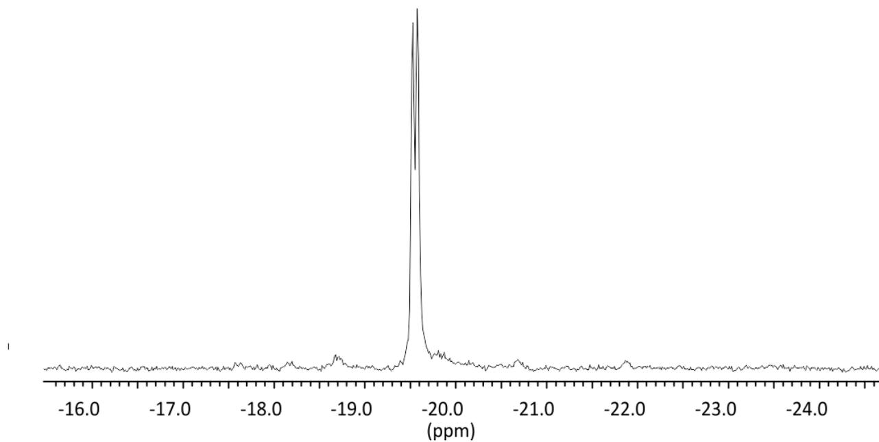
Figure S18.  $^{31}\text{P}\{^1\text{H}\}$  NMR spectrum (121.5 MHz,  $\text{C}_6\text{D}_6$ , 298 K) of the reaction product (5) of 2a' with 1 equiv of  $\text{tPrN}=\text{C}(\text{PPh}_2)\text{-N(H)tPr}$ .
