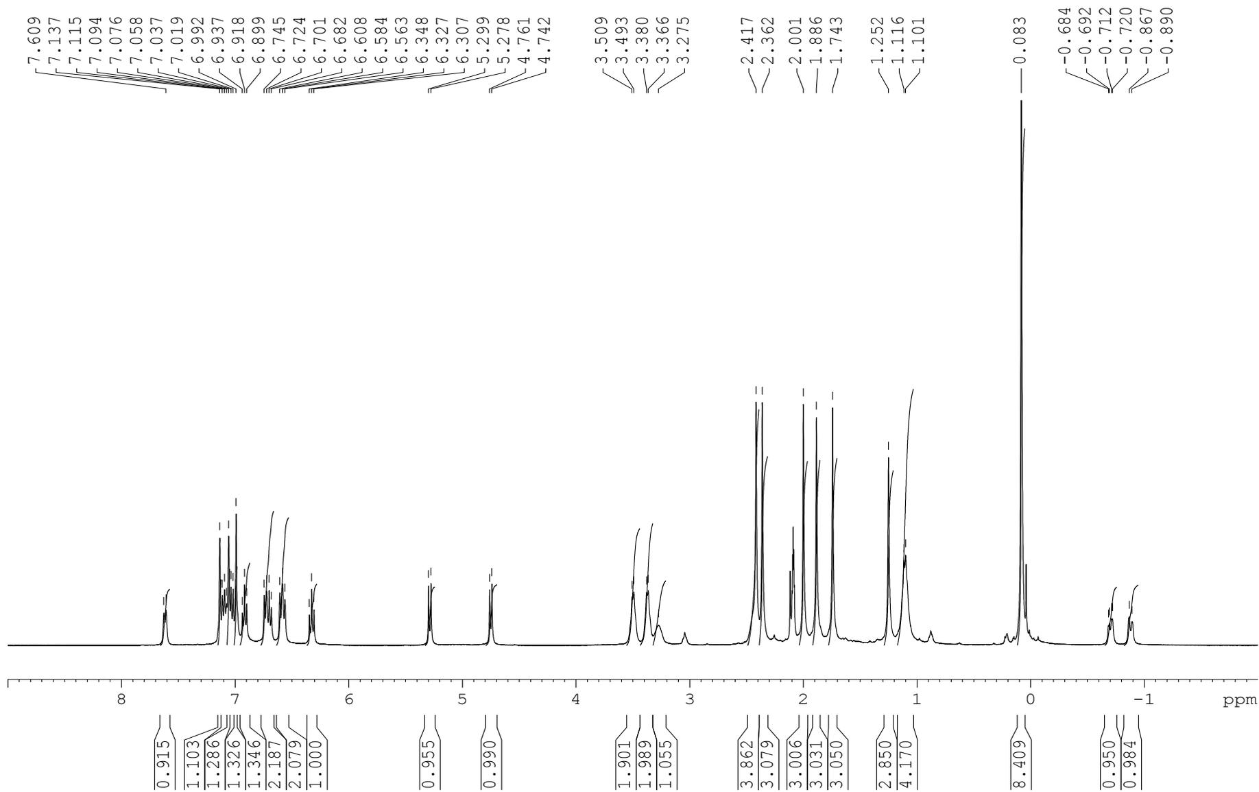
Figure S10.  $^1\text{H}$  NMR spectrum (400 MHz, toluene- $d_8$ , 233 K) of the reaction product (3) of 2a' with 1 equiv of  $\text{B}(\text{C}_6\text{F}_5)_3$ .
