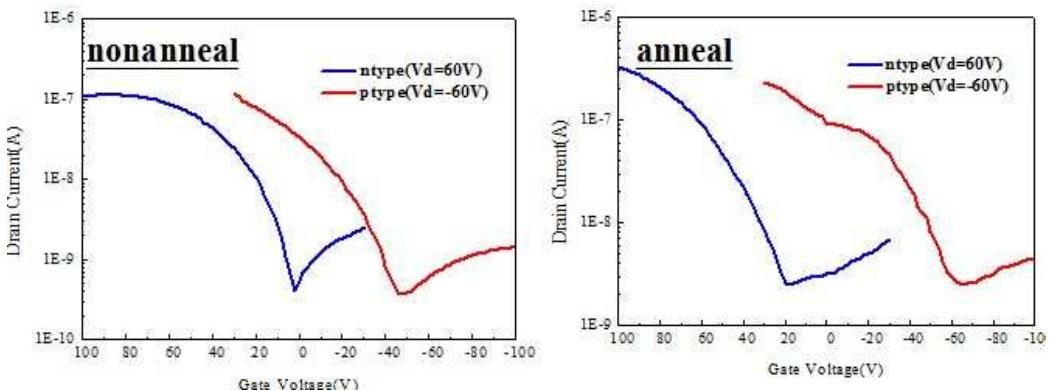
**Figure S13.** The transfer characteristic of physical blend of PCTT-g-P3HT and PNDICTT<sub>91</sub>.
