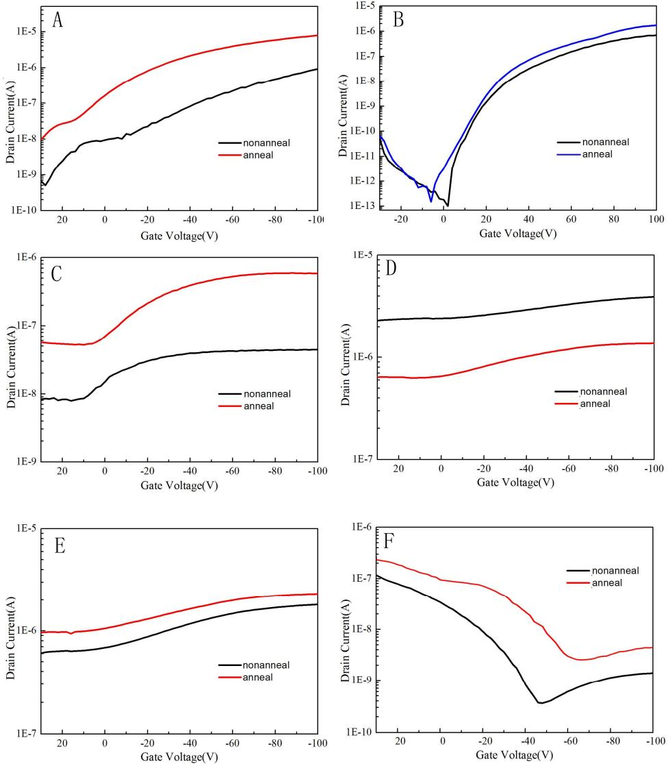
**Figure S12.** The transfer characteristic of PCTT-g-P3HT (A), PNDICTT<sub>91</sub> (B), PNDICTT<sub>91</sub>-g-P3HT(C), PNDICTT<sub>73</sub>-g-P3HTa(D), PNDICTT<sub>55</sub>-g-P3HT (E), and physical blend of PCTT-g-P3HT and PNDICTT91 (F).
