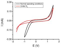
Figure 3. Electrodymanic profiles obtained with 3 electrodes fabricated with 12 layers of protein adsorbed/pyrolyzed. Conditions: 1.0 mM  $K_3Fe(CN)_6$  in 0.1 M NaH<sub>2</sub>PO<sub>4</sub>/Na<sub>2</sub>HPO<sub>4</sub> buffer + 0.1 M KCI, pH = 7.4, scan rate: 100 mV·s<sup>-1</sup>.
