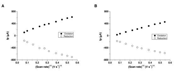
Figure 1. Dependence of the peak current (Ip) as a function of the square root of the scan rate obtained with the OTCE fabricated with 12 layers of protein adsorbed/pyrolyzed for  $K_3Fe(CN)_6$  (A) and  $Ru(NH_3)_6Cl_3$  (B). Conditions: 1 mM for each electrochemical couple in 0.1 M  $NaH_2PO_4/Na_2HPO_4$  buffer + 0.1M KCI, pH = 7.4.
