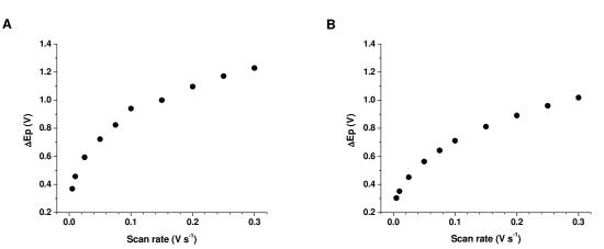
Figure 2. Dependence of the peak potential difference ( $\Delta$ Ep) as a function of the scan rate obtained with the OTCE fabricated with 12 layers of protein adsorbed/pyrolyzed for K<sub>3</sub>Fe(CN)<sub>6</sub> (A) and Ru(NH<sub>3</sub>)<sub>6</sub>Cl<sub>3</sub> (B). Conditions: 1 mM for each electrochemical couple in 0.1 M NaH<sub>2</sub>PO<sub>4</sub>/Na<sub>2</sub>HPO<sub>4</sub> buffer + 0.1M KCl, pH = 7.4.
