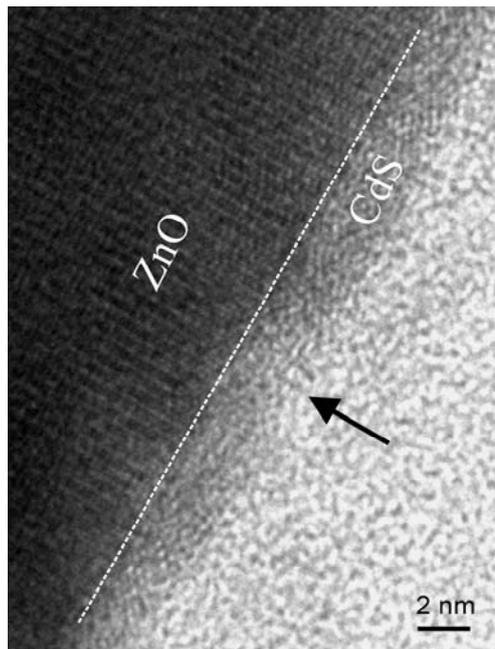
**Figure S2.** HRTEM image of a ZnO/CdS-core/shell nanorod with  $L = 3$  nm. The arrow shows the ZnO region that was not well passivated by CdS due to the quite thin CdS layer formed.
