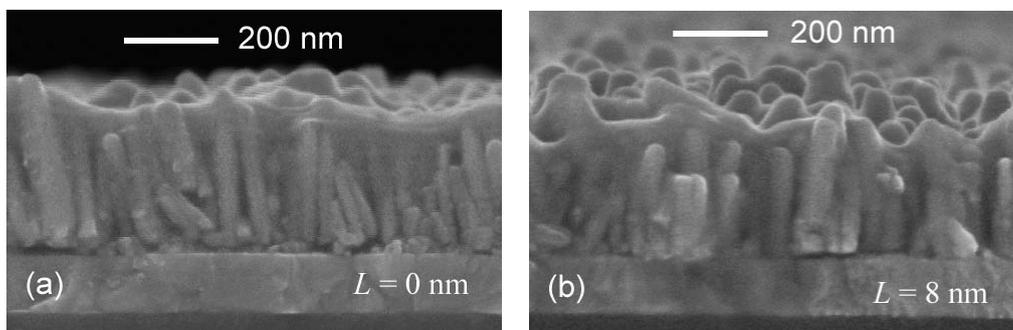
**Figure S3.** SEM images of MEH-PPV/ZnO-NA (a) and MEH-PPV/ZnO-CdS-NA (b) composite films, showing the good polymer infiltration in the interspaces between nanorods.
