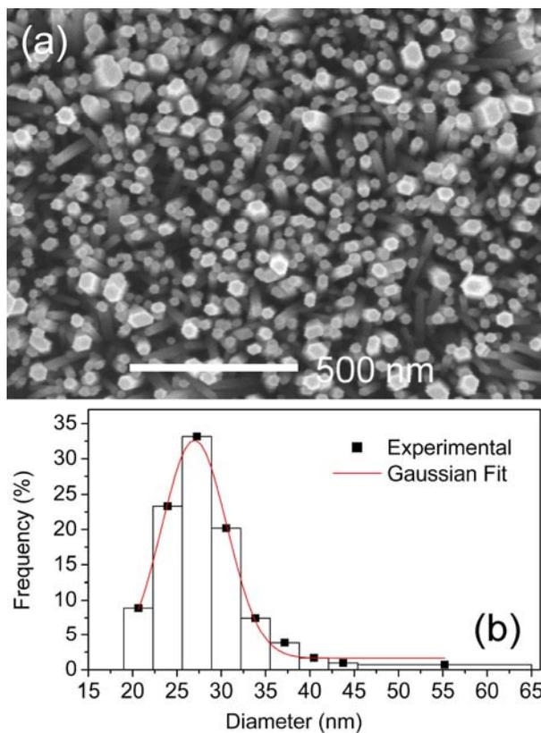
**Figure S4.** (a) SEM image of ZnO-NA, (b) Statistical histogram showing distribution of ZnO nanorod diameter in the ZnO-NA. ZnO nanorods had a number density of about  $420/\mu\text{m}^2$  and statistically an averaged diameter of ca. 28 nm.
