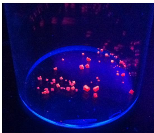
Figure S4. A photograph of MTP after immersion in 40 mM \text{EuNO}_3 \cdot 6\text{H}_2\text{O} aq. under UV light (365 nm) irradiation.
