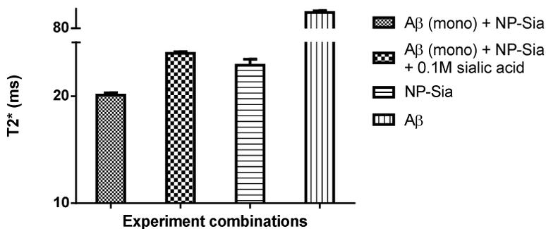
**Figure S4.** MRI generated T2\* values of NP-Sia/Aβ binding. NP-Sia (0.1 mg/mL) incubated with Aβ monomers (30 μM) and also in the presence of free sialic acid (0.1 M). The error bars represent the standard deviation of three measurements.
