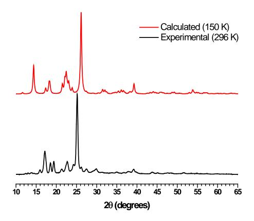
**Figure S7.** Comparison of calculated and experimental X-ray powder diffraction patterns for crystals of (**BI**/H<sup>+</sup>)<sub>2</sub> (**TA**<sup>-2</sup>) grown from DMSO.
