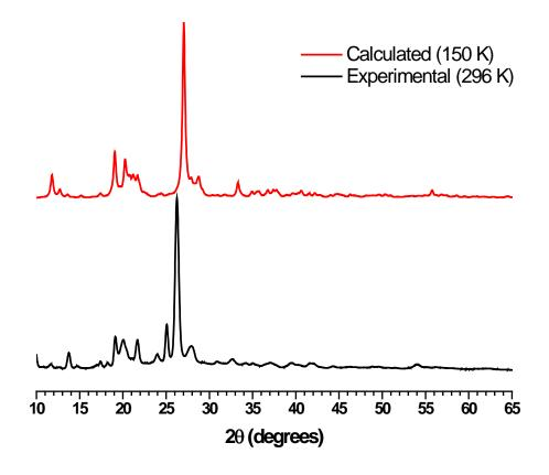
**Figure S8.** Comparison of calculated and experimental X-ray powder diffraction patterns for crystals of  $(BI/H^+)_2$   $(TMA/H^{-2}) \cdot H_2O$  grown from DMSO.
