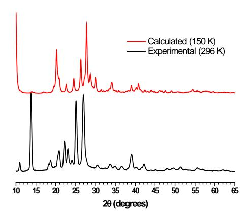
**Figure S6.** Comparison of calculated and experimental X-ray powder diffraction patterns for crystals of  $(\mathbf{BI/H^+})_2 (\mathbf{FA^{-2}}) \cdot 4H_2O$  grown from DMSO.
