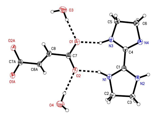
**Figure S2.** Thermal atomic displacement ellipsoid plot of the structure of crystals of  $(\mathbf{BI/H}^+)_2$   $(\mathbf{FA}^{-2}) \cdot 4H_2O$  grown from DMSO. The ellipsoids of non-hydrogen atoms are drawn at the 50% probability level, and hydrogen atoms are represented by a sphere of arbitrary size. Hydrogen bonds are shown as dotted lines. Atoms labelled with a suffix A are generated by the symmetry operation -x, -y+1, -z.
