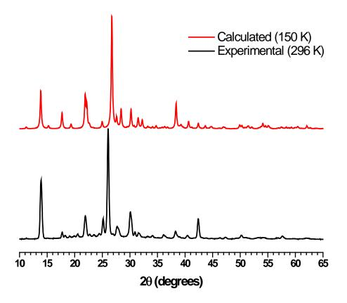
**Figure S5.** Comparison of calculated and experimental X-ray powder diffraction patterns for crystals of  $(\mathbf{BI/H_2}^{+2})$   $(\mathbf{OA}^{-2})$  grown from DMSO.
