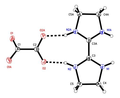
**Figure S1.** Thermal atomic displacement ellipsoid plot of the structure of crystals of (**BI**/H<sub>2</sub><sup>+2</sup>) (**OA**<sup>-2</sup>) grown from DMSO. The ellipsoids of non-hydrogen atoms are drawn at the 50% probability level, and hydrogen atoms are represented by a sphere of arbitrary size. Hydrogen bonds are shown as dotted lines. Atoms labelled with a suffix A are generated by the symmetry operation -x+1, y, -z+3/2.
