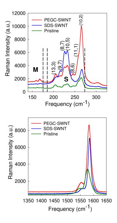
**Figure S3.** Raman spectra obtained for PEGC-SWNT, SDS-SWNT, and pristine samples with a 785 nm excitation laser line.
