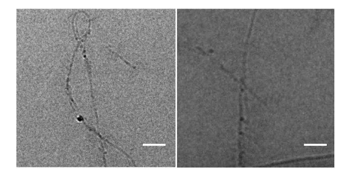
**Figure S2.** Sample transmission electron microscope (TEM) images prepared from dilute solution of PEGC-SWNT sample. Some circular features are present on nanotube surfaces. These features can be attributed to adsorbed PEGC molecules. Dark spots could be a result of aggregation of PEGC on SWNT surface upon drying during sample preparation. TEM images were collected with JEOL JEM-100 CX II transmission electron microscope. The scale bar corresponds to 100 nm.
