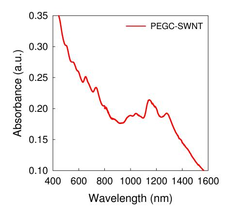
Figure S1. PEGC-SWNT absorption between 400 and 1600 nm.
