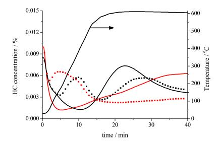
**Figure S4.** Simulated cold start test for the different zeolites,  $CO_2$  evolution during the third CST. Conditions: 100 ppmv propene, 90 ppmv toluene, 1% v/v  $O_2$ , 10% v/v  $H_2O$  and Ar balance. GHSV= 10000 h<sup>-1</sup>. Black line represents H-ZSM-5  $CO_2$  concentration profile, red represents CuH-ZSM-5(1), black dotted line presents CuH-ZSM-5(2) and red dotted line represents CuH-ZSM-5(3).
