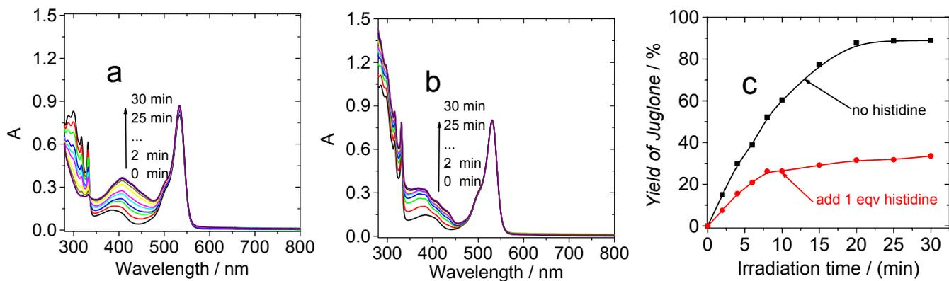
**Figure S88.** UV/Vis absorption spectral changes for the photooxidation of DHN. (a) **B-1** as a photocatalyst. (b) **B-1** as sensitizer, with addition of 1.0 eqv. histidine. (c) Plots of chemical yields as a function of irradiation time.  $c[\text{sensitizers}] = 1.0 \times 10^{-5} \text{ M}$ .  $c[\text{DHN}] = 1.0 \times 10^{-4} \text{ M}$ . light intensity: 20 mW/cm<sup>2</sup> (MeOH, 20 °C).
