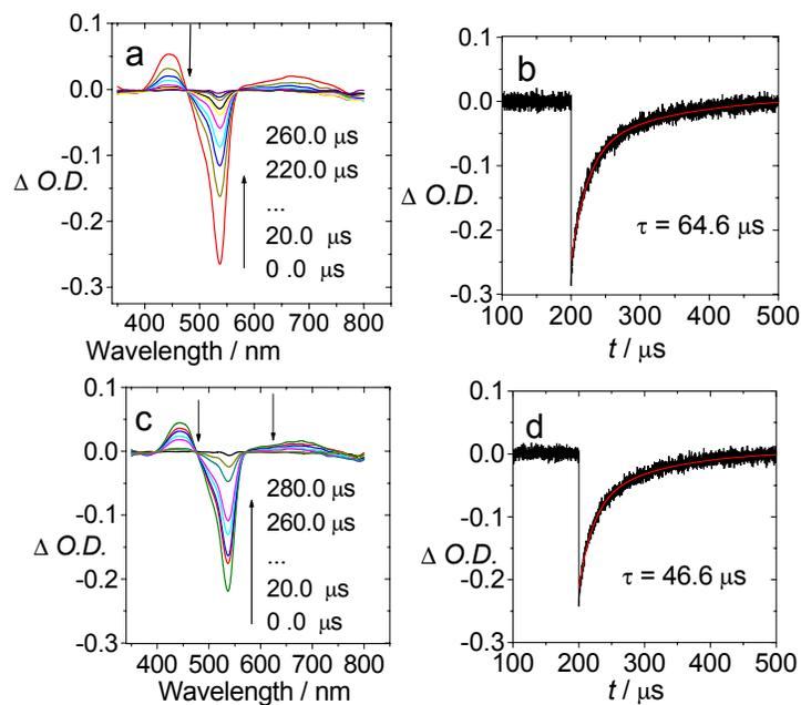
**Figure S84.** Nanosecond time-resolved transient difference absorption of **B-1**. (a) transient absorption difference spectra of **B-1** and (b) decay trace at 540 nm. Transient difference absorption of **B-1** in the presence of 100 eq benzylamine, (c) transient absorption difference spectra and (d) decay trace at 540 nm. In deaerated CH<sub>3</sub>CN.  $1.0 \times 10^{-5}$  M,  $\lambda_{\text{ex}} = 532$  nm, 25 °C.
