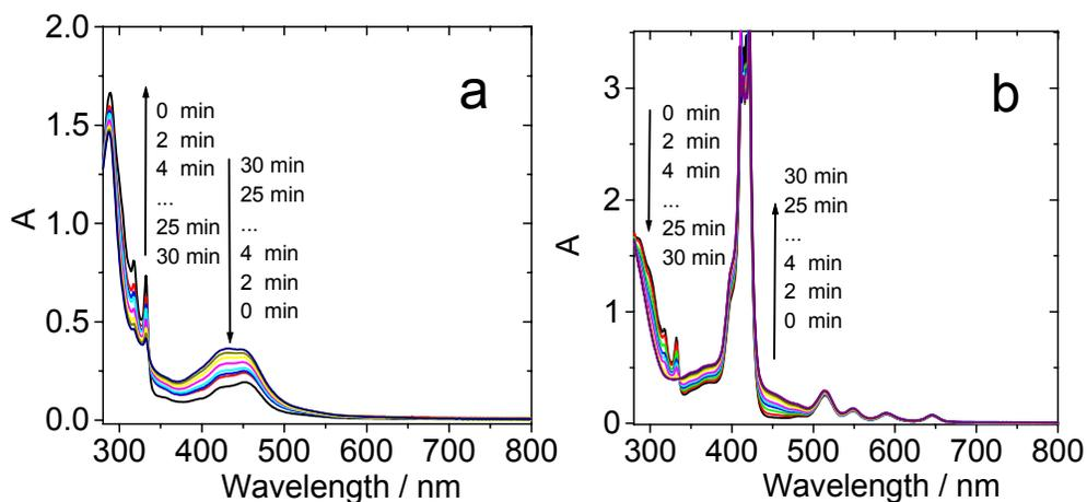
**Figure S86.** UV-vis absorption spectral changes for the photooxidation of DHN. (a) **Ru(bpy)<sub>3</sub>[PF<sub>6</sub>]<sub>2</sub>** as a sensitizer. (b) **TPP** as sensitizer.  $c[\text{sensitizers}] = 1.0 \times 10^{-5} \text{ M}$ .  $c[\text{DHN}] = 1.0 \times 10^{-4} \text{ M}$ . light intensity:  $20 \text{ mW/cm}^2$  ( $\text{CH}_2\text{Cl}_2/\text{MeOH}$ , 9:1, v/v,  $20^\circ\text{C}$ ).
