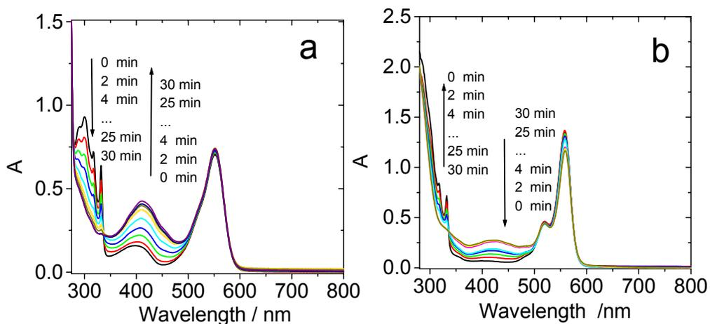
**Figure S85.** UV-vis absorption spectral changes for the photooxidation of DHN. (a) **B-3** as a sensitizer. (b) **B-4** as sensitizer.  $c[\text{sensitizers}] = 1.0 \times 10^{-5} \text{ M}$ .  $c[\text{DHN}] = 1.0 \times 10^{-4} \text{ M}$ . light intensity:  $20 \text{ mW/cm}^2$  ( $\text{CH}_2\text{Cl}_2/\text{MeOH}$ , 9:1, v/v,  $20^\circ\text{C}$ ).
