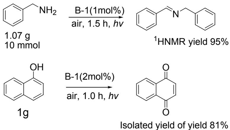
**Scheme S1.** Scale-up of the photocatalytic reactions. Benzylamine (10 mmol), **B-1** (0.1 mmol, 1 mol %), solvent: acetonitrile (150 mL), in air,  $\lambda > 380 \text{ nm}$  ( $20 \text{ mW/cm}^2$ ),  $20 \text{ }^\circ\text{C}$ . Naphthol (7.0 mmol, 1.0 g), **B-1** (5.0 mol%), were mixed in co-solvent ( $\text{CHCl}_3/\text{Methol}=4/1$ , v/v). The mixture was irradiated with 35 W Xe lamp ( $\lambda > 385 \text{ nm}$ , light powder density:  $30 \text{ mW/cm}^2$ ).
