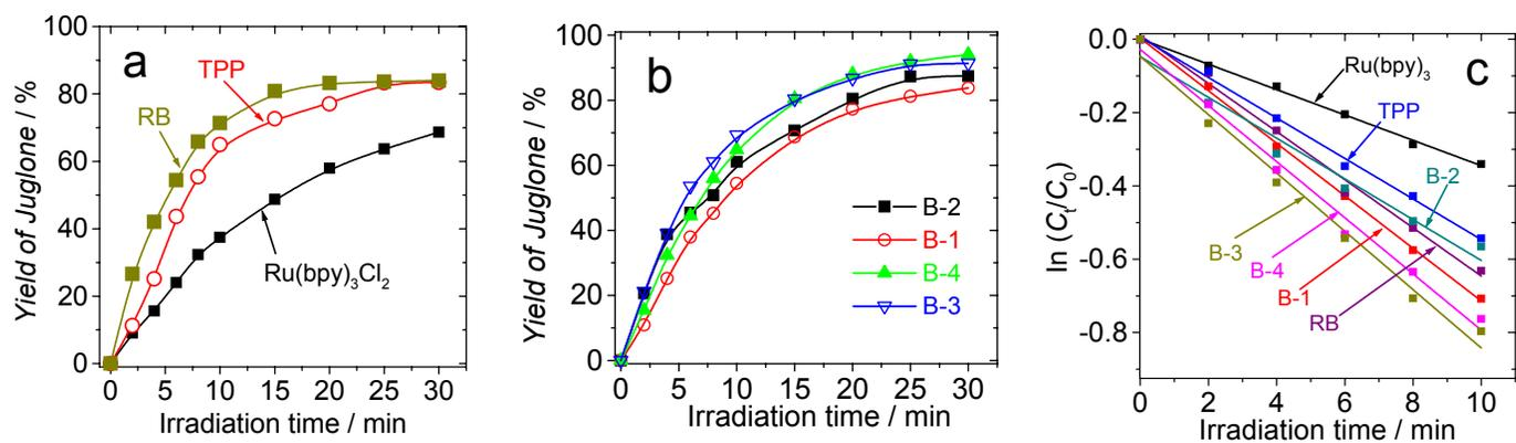
**Figure S87.** Photooxidation of DHN with triplet photosensitizers. (a) and (b) plots of chemical yields as a function of irradiation time. (c) Plots of  $\ln(C_t/C_0)$  vs. irradiation time ( $t$ ) for the photooxidation of DHN (CH<sub>2</sub>Cl<sub>2</sub>/MeOH, 9:1, v/v, 20 °C)
