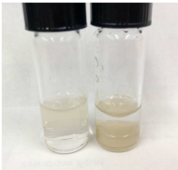
Figure S6. Photograph of silver nanospheres before and after phase transfer. Top layer: water, bottom layer, chloroform. Note that the sample on the right is 5 times more concentrated than the one on the left.
