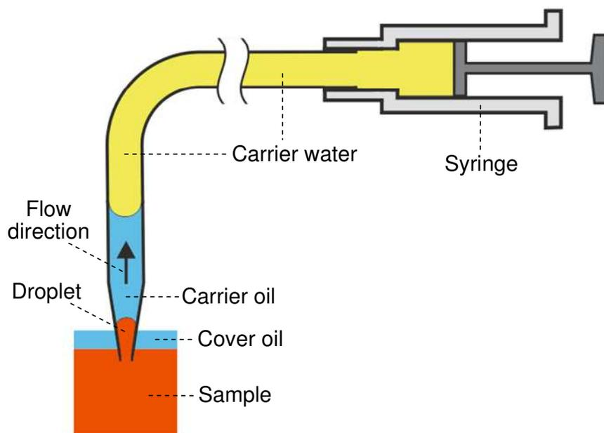
Figure S3. Schematic diagram showing the liquids in the capillary-syringe pump module. The syringe and capillary are filled with carrier water instead of oil to minimize the thermal expansion and contraction of the liquid filled in them. A 10 nL plug of carrier oil is filled in the tip of the capillary to segment the aspirated droplet from the carrier water.
