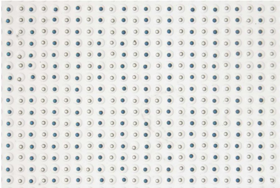
Figure S7. A CCD image of an array of 384, 480-pL droplets with different dyes for showing the ability of the SODA system in generation large number of droplets.
