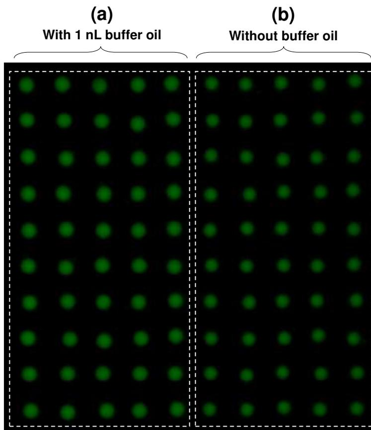
Figure S4. Fluorescent image of droplet array including 50 droplets generated with 1-nL buffer oil (a) and 50 droplets without the buffer oil (b), respectively. The set droplet volume in both (a) and (b) experiments is 990 pL. An evident decrease in droplet volumes (ca. 300 pL) can be observed in (b) compared with (a) due to the influence of the syringe pump mechanical backlash.
