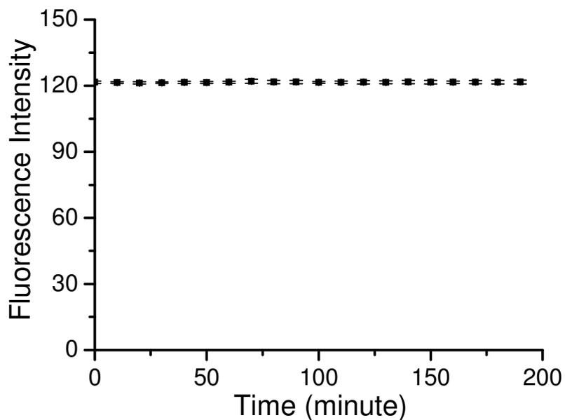
Figure S5. Testing of the effect of oil in reducing evaporation of water in droplets by monitoring the fluorescence intensity of three 480-pL droplets for over three hours using sodium fluorescein (10  $\mu\text{M}$ ) as a model sample.
