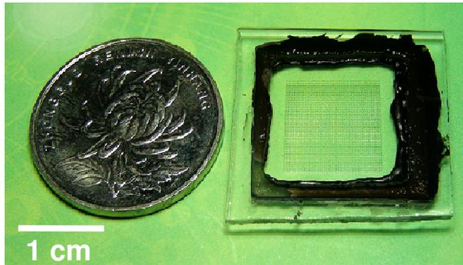
Figure S1. Images of the microchip with picowell array. The picowell array was fabricated at a density of 1600 droplets/cm<sup>2</sup>.
