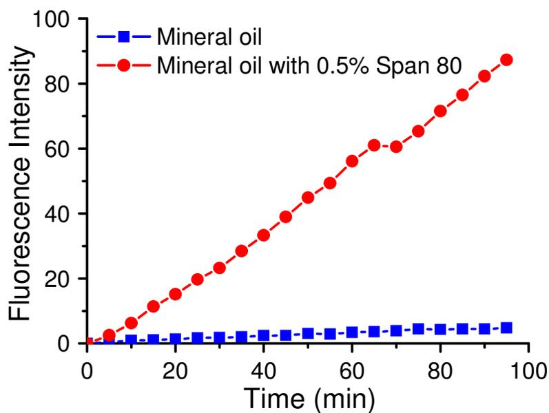
Figure S6. Results of enzyme activity measurement for caspase-1 in droplets using mineral oil with and without surfactant Span 80 (0.5%, v/v). Droplet volume: 1.98 nL; enzyme concentration: 6 mU/ $\mu\text{L}$ ; substrate concentration: 20  $\mu\text{M}$ .
