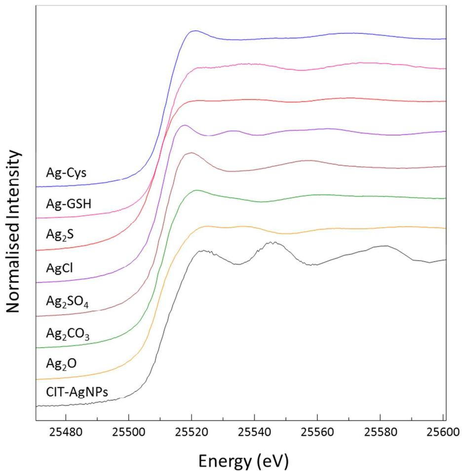
**Figure S4.** Raw XANES profiles (pre-normalisation) of all samples showing the different absorbance magnitude after exposure, suggesting some loss of silver (as  $\text{Ag}^+$ ,  $\text{AgNP}$ , or otherwise) from the surface. Note that the pre-exposure variability in the AgNPs attachment density is *ca.* 10 %.
