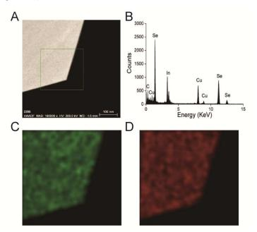
Figure S2. TEM characterization of In<sub>2</sub>Se<sub>3</sub> flakes. (A) TEM image of an In<sub>2</sub>Se<sub>3</sub> flake. (B) Typical EDX spectrum of the In<sub>2</sub>Se<sub>3</sub> flake. The Cu and C signals come from the TEM grid. (C, D) In and Se element maps of the corresponding In<sub>2</sub>Se<sub>3</sub> flake, respectively.
