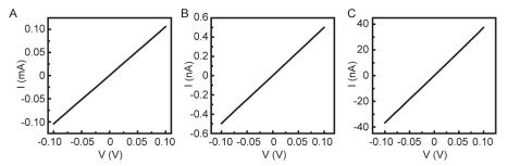
Figure S3. Phase transition of 2D  $In_2Se_3$  flakes induced by annealing and electron beam irradiation: (A) Two-probe I-V measurement of an  $In_2Se_3$  flake with a superlattice structure; (B) Two-probe I-V curve of the same  $In_2Se_3$  flake after annealing; (C) Two-probe I-V curve of the same  $In_2Se_3$  after annealing and electron beam irradiation.
