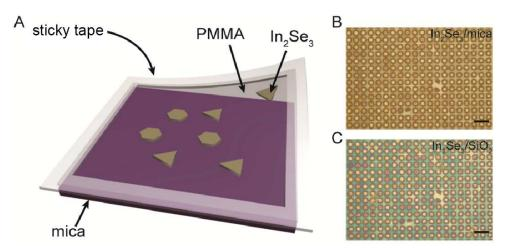
Figure S1. (A) Schematic diagram for the PMMA-mediated transfer technique. (B, C) Optical images of In<sub>2</sub>Se<sub>3</sub> flakes before and after transfer, respectively. Scale bars: 20 µm.
