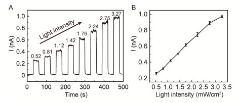
Figure S4. (A) Photocurrent of  $In_2Se_3$  flakes as a function of incident light density. (B) The output photocurrent change with incident light density.
