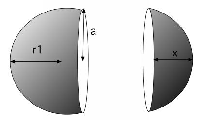
To determine A<sub>111</sub>, we note that the radius of the white circular facetted region,  $a_{111} = [(2r_1x)-x^2]^{1/2}$ . Thus,  $E_2 = \gamma_s (4\pi r_1^2) + 2\pi \gamma_{s111} [(2r_1x) - x^2] + (4/3\pi r_1^3 G_{vs})$ .
