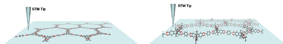
Scheme 1. Illustration for tiled (left) and vertical (right) alignments of COF structures on STM substrates.
