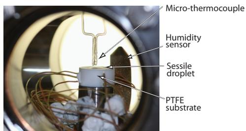
**Figure S1.** A sessile droplet of ethanol resting on the PTFE substrate inside the evaporation chamber may be seen in the photograph.
