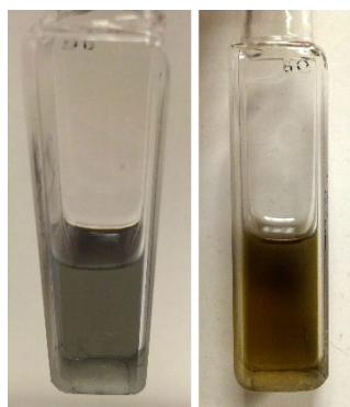
Figure S7. Coloration of ZnO nanocrystal suspensions when exposed to UV illumination in the presence of \text{Li}[\text{Et}_3\text{BH}] or \text{Li}[\text{Me}_2\text{NBH}_3] .
