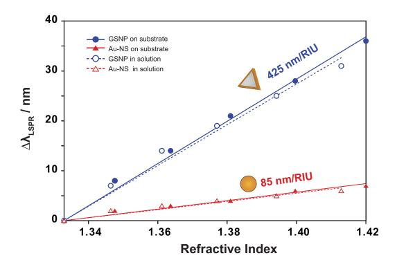
**Figure S3:** Comparison of bulk refractive index sensitivity for GSNPs and gold nanospheres immobilized on a substrate and in solution. No difference in sensitivity can be observed. Bulk refractive index sensitivity for dispersed nanoparticles was determined by mixing 10  $\mu$ l of highly concentrated nanoparticles together with 100  $\mu$ l of various sucrose solutions (0-50%, w/w)
