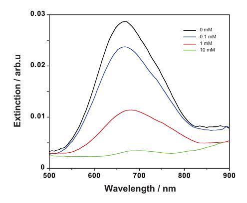
**Figure S4:** UV-VIS spectra of GSNPs exposed to  $H_2O_2$  at different concentrations. GSNPs were immobilized in a microtiter plate using PEI/PSS/PAH with the protocol described in the methods section. Various concentration of hydrogen peroxide was added to the particles, incubated for 15 min followed by rinsing and finally, extinction spectra were recorded using UV-Vis spectroscopy.
