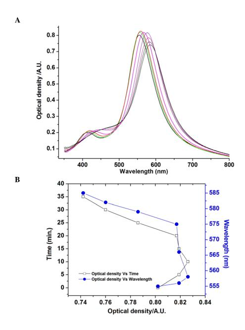
**Figure S1:** A) Typical SPR band evolution during 35 min edge gold-coating. B) Close look of SPR band evolution in A. The SPR band red-shifted ~30 nm after edge-gold coating.
