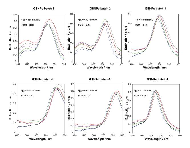
**Figure S2:** UV-VIS spectra for six different batches of dispersed GSNPs in various concentrations of sucrose (0-50%). Bulk RI sensitivities ( $\eta_B$ ) and FOM-values are reported for each batch.
