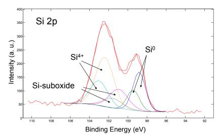
Figure S1. X-ray photoelectron spectrum Si 2p of dry silicon nanocrystal powder.
