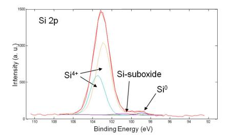
Figure S2. X-ray photoelectron spectrum Si 2p of silicon nanocrystal powder stored in water for about 3 days.
