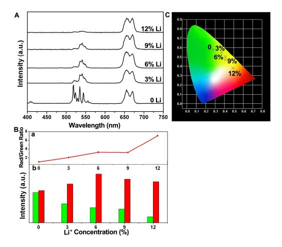
**Figure S3**. UC luminescence spectra of  $GdF_3:15\%Yb^{3+},1\%Er^{3+},y\%Li^+$  (y=0, 3, 6, 9 and 12) under 980 nm excitation (A); the red/green ratio (a) and integral intensity (b) of the green and red colors with different  $Yb^{3+}$ -doped concentration (B). CIE chromaticity diagram of  $GdF_3:15\%Yb^{3+},1\%Er^{3+},y\%Li^+$  (y=0, 3, 6, 9 and 12) under 980 nm excitation (C).
