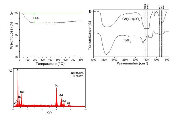
Figure S1. TG curve (A), FT-IR (B) and EDS (C) of the  $GdF_3$  hollow spheres.
