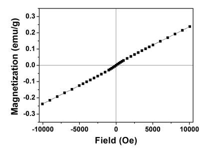
Figure S4. Magnetization as a function of the applied field for GdF<sub>3</sub> hollow spheres.
