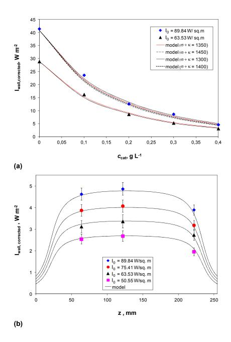
**Figure S4.** Forward photon flux emerging from the outer wall of PR1. (a) At different TiO<sub>2</sub> powder loadings and different levels of irradiance, at  $z^* = 0.5$ . Lines are the fitting of SFM with  $\omega = 0.8617$ , symbols are mean values of several measurements. (b) At different positions along the axial direction varying the irradiance. Lines are the fitting of SFM with  $\omega = 0.8617$ . [TiO<sub>2</sub>] = 0.4 g/L.
