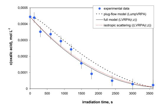
**Figure S5.** Results of the 5odelling of the photocatalytic oxidation of oxalic acid in PR1 with different model assumptions. pH = 4,  $[TiO_2] = 0.4 \text{ g/L}$ ;  $I_0 = 89.84 \text{ W m}^{-2}$ .
