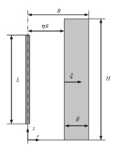
**Figure S3.** Schematic representation of the geometry of the annular photocatalytic reactor (reproduced from Toepfer et al.<sup>1</sup>).
