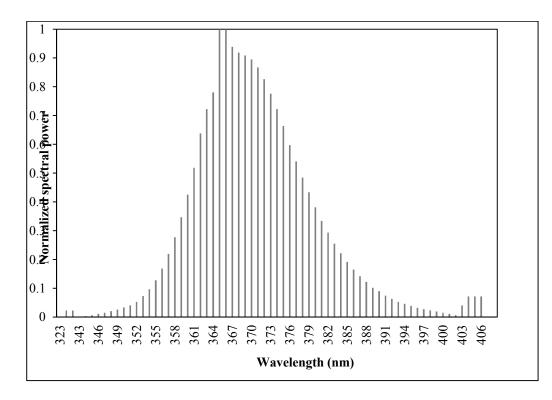
**Figure S1.** Emission spectrum for blacklight blue fluorescent lamps (Philips blacklight-blue TL 8W/08 F8 T5/BLB lamp).
