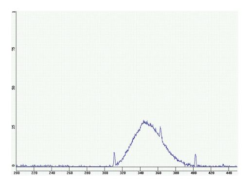
**Figure S2.** Emission spectrum for UVP Pen-Ray® mercury discharge lamp (model 90-0019-04) provided by UVP.
